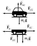
From consideration of the vertical forces in the individual free-body diagrams, it is apparent that the normal force on each object is equal to its weight. This leads to the conclusion that
