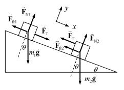
considered,  $m_1$  will move more distance down the plane upon release than block  $m_2$ . The cord will go slack almost immediately after the blocks are released, and the blocks revert to the original free-body diagram. The conclusion is that the accelerations in this part of the problem are the same as they would be in part (*a*):
