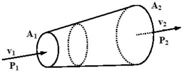
Mass entering the streamtube = Volume \* Density =  $A_1(v_1t)*\rho$ Momentum entering the streamtube = Mass\*Velocity =  $A_1(v_1t)\rho*v_1$
