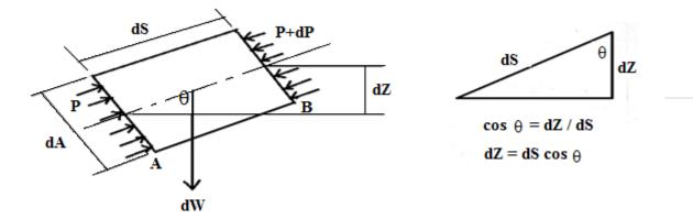
ds, dA: length and cross sectional area of the fluid element.
