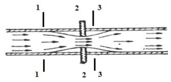
For ideal fluid, applying Bernoulli's equation between sections (1) and (2) representing the pipe and orifice respectively,
