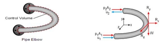
$\label{eq:FT} \underline{\textit{In general}}, \qquad \qquad F_T = F_B + F_W + F_P = \rho \; Q \; (v_{out} - v_{in})$
