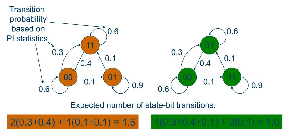
State encoding can be selected using a power-based cost function.
