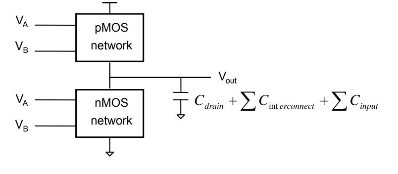
$$P_{avg} = \frac{1}{T} \left[ \int_{0}^{T/2} V_{out} \left( -C_{load} \frac{dV_{out}}{dt} \right) dt + \int_{T/2}^{T} \left( V_{DD} - V_{out} \right) \left( C_{load} \frac{dV_{out}}{dt} \right) dt \right]$$
