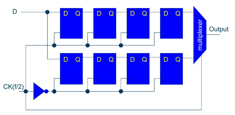
Flip-flops are operated at full voltage and half the clock frequency.
