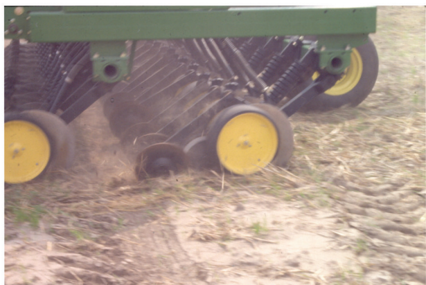
Figure 5. A single-disk opener operating in wheat stubble.
