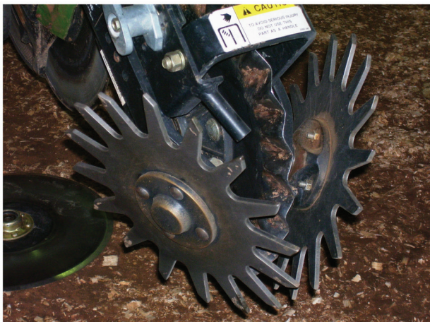
Figure 19. A combination coulter/row cleaner.
