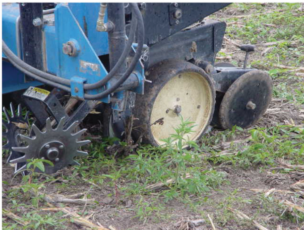
Figure 18. A spoke-type row cleaner on a Kinze planter.
