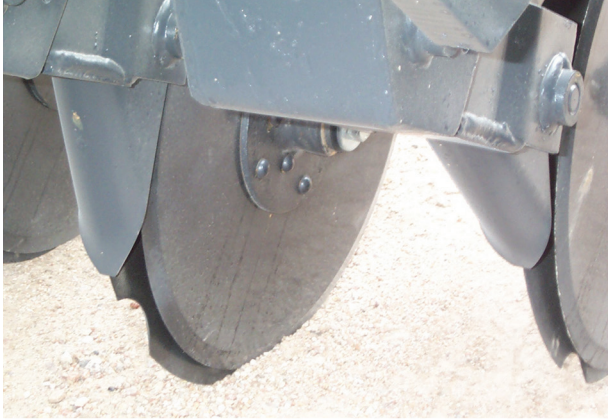
Figure 9. A double disk opener on a no-till drill with staggered disks and a notched leading blade.
