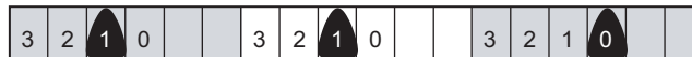
Fig. 4-8. OPPM with N = 3 and M = 2 has six chips per two bits. The four possible starting positions for three-chip-wide pulses are indicated. Modulation of message 101001 is shown.
