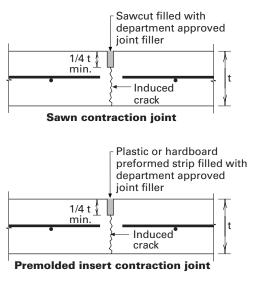
Figure 5.15. Control (contraction) joint.
