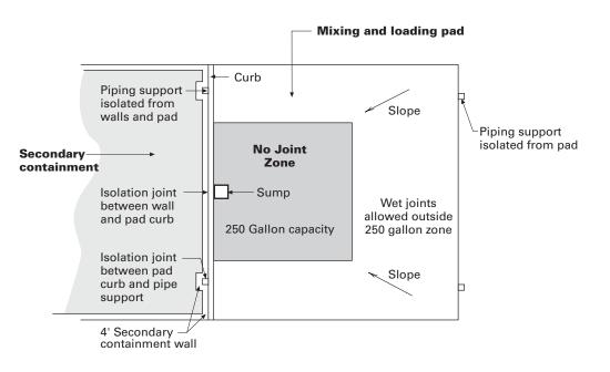
Figure 5.9. Common Joints in mixing and loading pad (side sump design). Note location of piping support outside mixing and loading pad.
