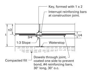
Figure 5.25. Floor construction joint with waterstop at bottom (wet joint).
