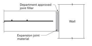
Figure 5.13. Isolation joint.
