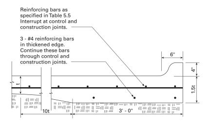
**Figure 5.4**. Concrete detail for mixing and loading pad floor with integral edge curb. (See table 5.4 for concrete thickness, t).
