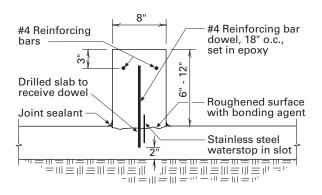
Figure 5.19. Retrofit curb-to-floor joint (dry or wet joint).
