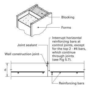
Figure 5.28. Wall construction joint (dry joint).
