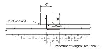
Figure 5.18. Interior curb-to-floor joint (wet joint).
