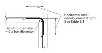
Figure 5.20. Reinforcing detail of a wall corner.
