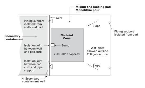
**Figure 5.10.** Common Joints in mixing and loading pad (side sump design). Note location of piping support outside secondary containment structure.
