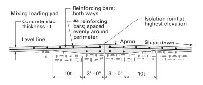
Figure 5.30. Floor Isolation joint (dry joint).
