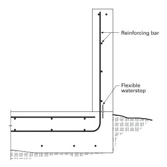
Figure 5.16. Wall-to-floor joint (wet joint).
