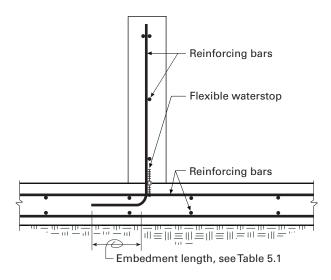
Figure 5.17. Interior wall-to-floor joint (wet joint).
