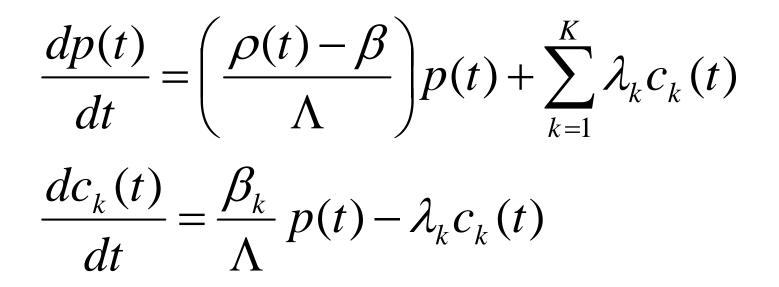
Most important assumption: Assumes that the perturbation introduced in the reactor affects only the amplitude of the flux and not its shape.
