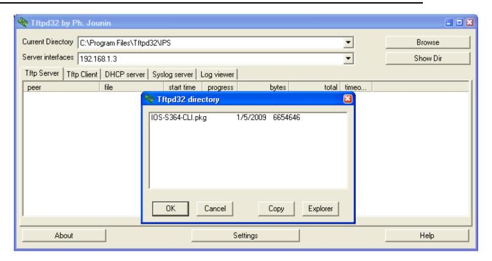
Step 3: Copy the signature package from the TFTP server to the router.
