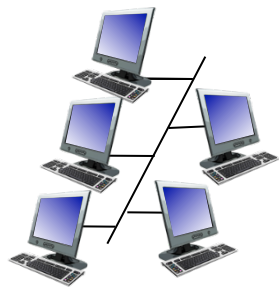
shared wire (e.g., cabled Ethernet)
