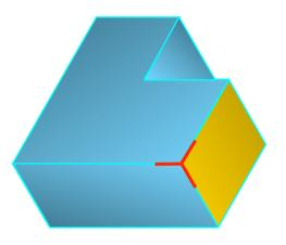
View point is looking up on the bottom of the object. View point is looking from the right (or left) of the object.
