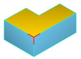
View point is looking down on the top of the object. Reverse axis isometric
