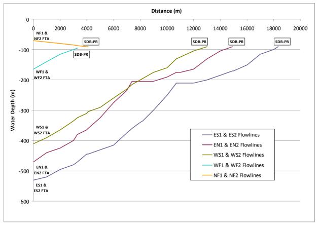
Figure 5.21 Approximate Flowline Lengths and Associated Seabed Profiles
