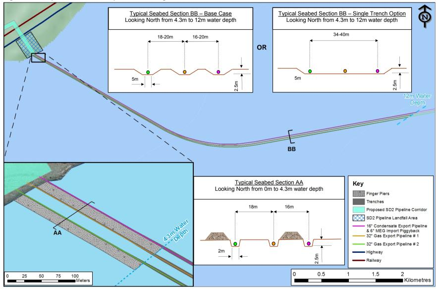
The works will commence with the construction of two temporary finger piers to allow construction plant access to the nearshore for trenching. The piers will be constructed by dumping aggregate in the shallow marine zone to achieve the required clearance above sea level<sup>16</sup>.
