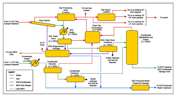
The SD2 onshore facilities are designed to incorporate two gas and condensate processing trains.
