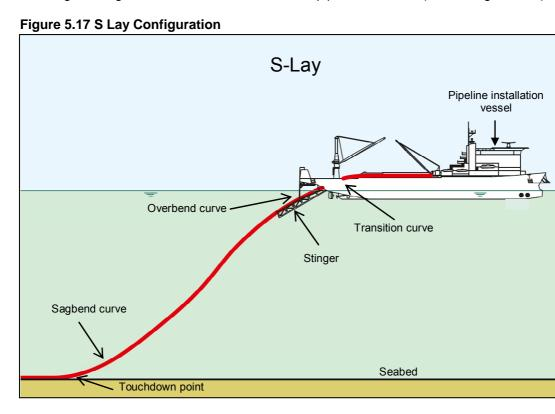
The 16" condensate line and 6" MEG line will be installed simultaneously. The 6" pipeline will be welded separately and the completed sections mechanically attached to the 16" pipeline using straps as it moves off the stern of the vessel.
