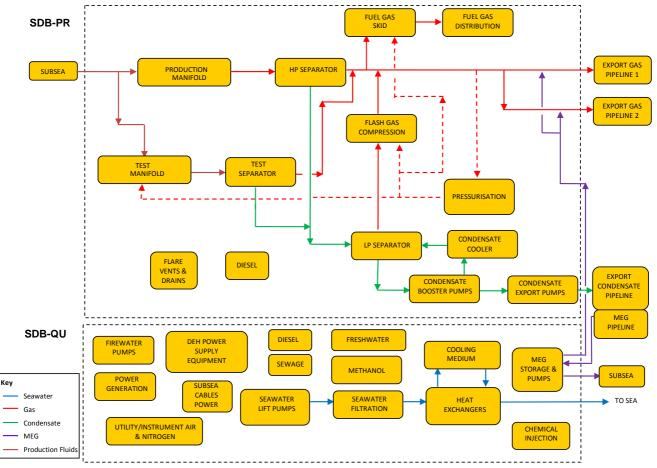
Figure 5.22 SDB-PR and SDB-QU Process and Utilities Systems
