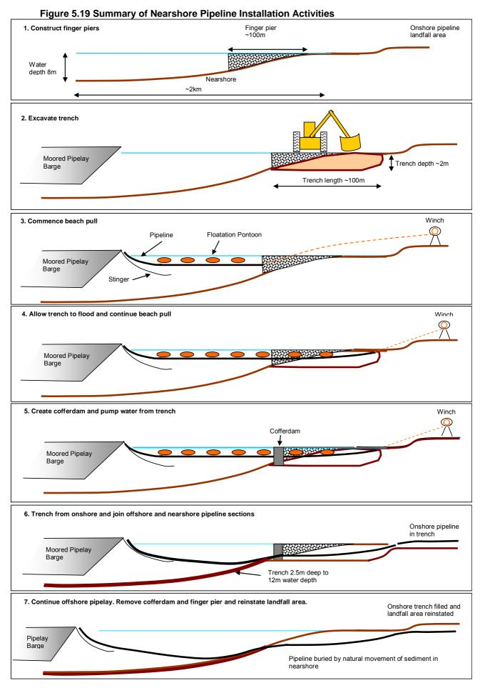
Based on current information, it is intended to dig the trenches to the 12m water depth contour by dredging the seabed using a cutter suction dredger (CSD). However, if further information obtained through ground truthing surveys to be performed in 2Q 2013 show the seabed and underlying material is not suited to the use of the CSD, alternative approaches may be considered.
