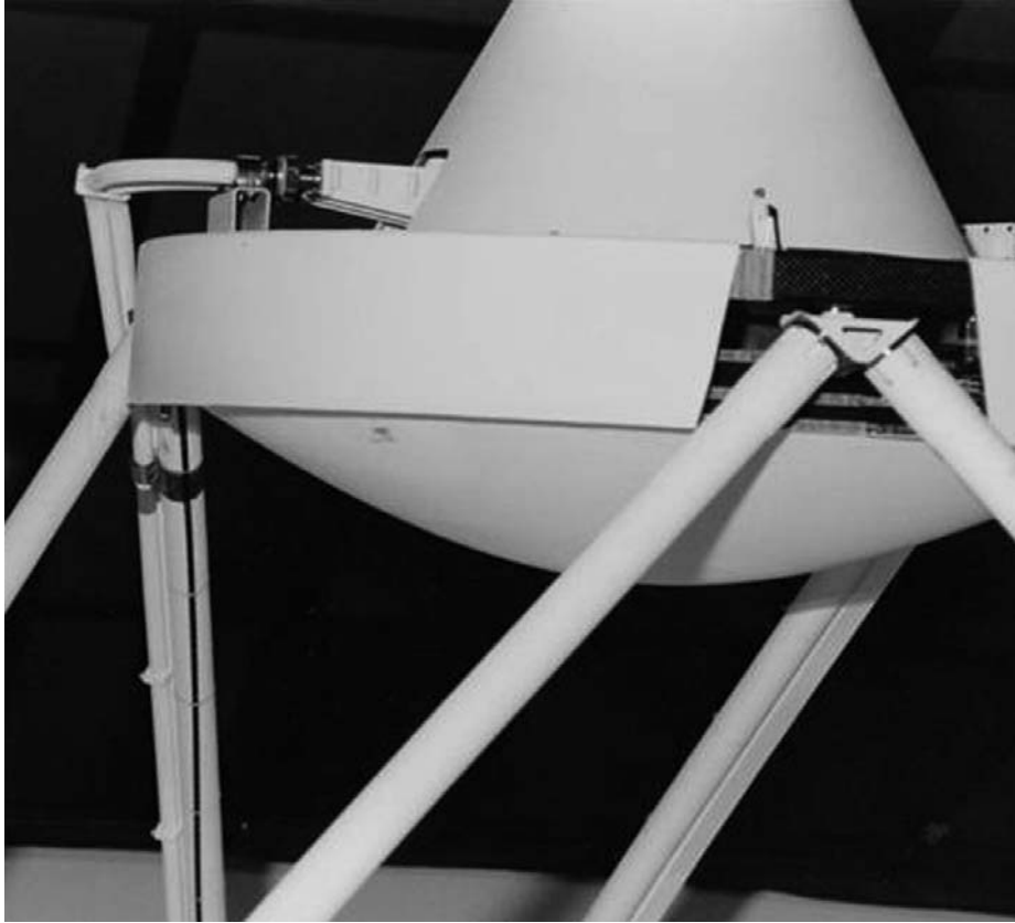
Fig. 5-38. Cassini FSS subreflector deck on HGA FM.
