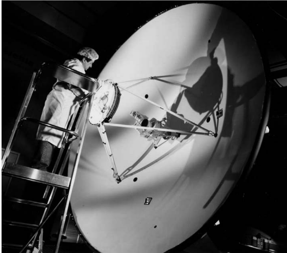
Fig. 5-35. Cassini HGA/LGA1 flight model.
