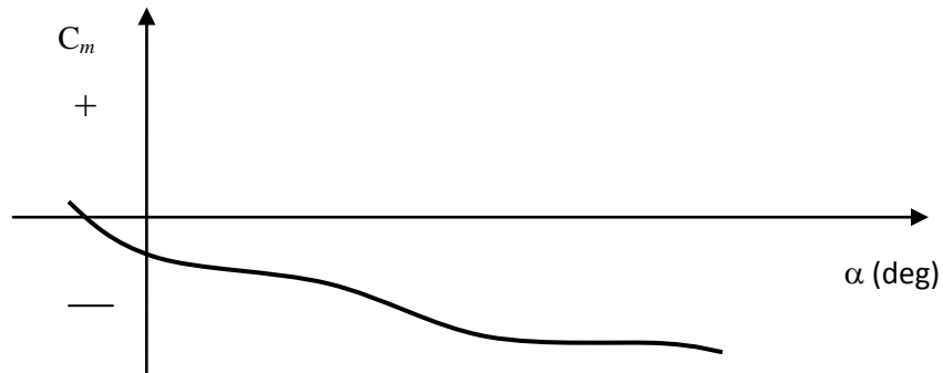
Figure 5.13. The variations of pitching moment coefficient versus angle of attack
