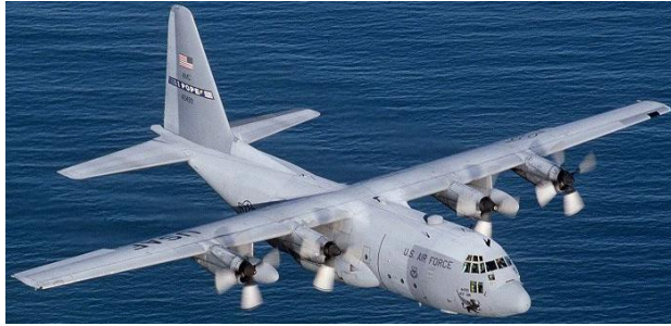
a. Cargo aircraft C-130 (high wing) (Photo courtesy of Tech. Sgt. Howard Blair, U.S. Air Force)
