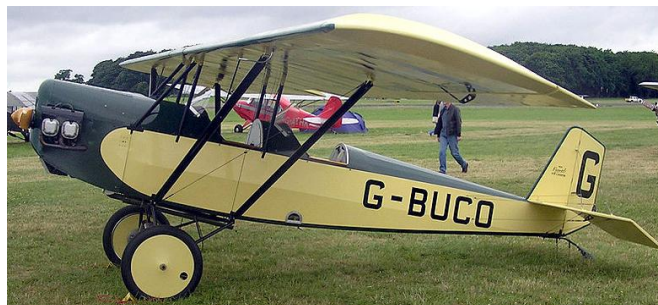
d. Home-built Pietenpol Air Camper (parasol wing) (Photo courtesy of Adrian Pingstone)
