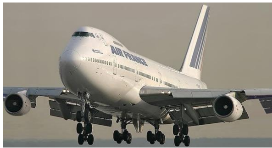
b. Passenger aircraft Boeing 747 (low wing) (Photo courtesy of Philippe Noret – AirTeamimages)
