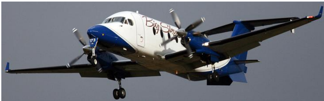
Figure 5. 61. The Hawker Beechcraft Beech King 1900D (note on winglets) (Photo courtesy of Prestwick 99)
