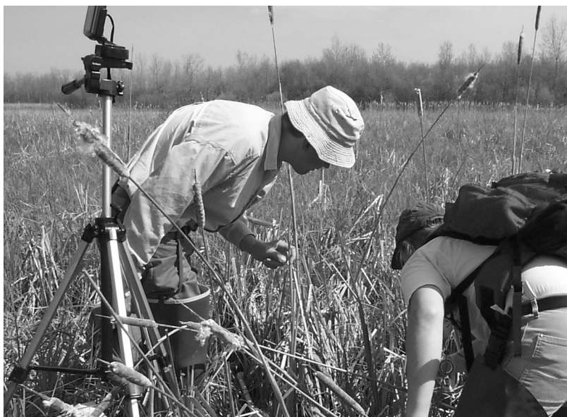
Figure 56-7 Field GPS unit attached to a tripod collects location data while field crew makes vegetation measurements.
