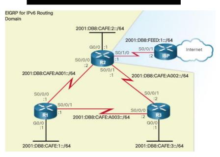
Unlike EIGRP for IPv4 which uses the network command, EIGRP for IPv6 is configured directly on the interface using the ipv6 eigrp autonomous-system interface configuration command.
