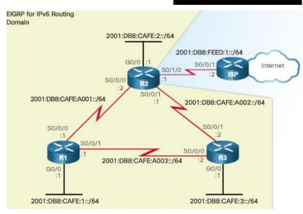
R3# show running-config <output omltted> ! interface GigabitEthernet0/0 ipv6 address 2001:DB8:CAFE:3::1/64 ! interface Serial0/0/0 ipv6 address 2001:DB8:CAFE:A003::2/64 clock rate 64000 ! interface Serial0/0/1 ipv6 address 2001:DB8:CAFE:A002::2/64
