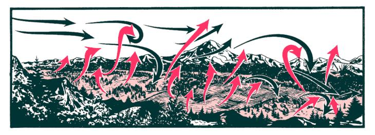
Thermal turbulence caused by surface heating is a mechanism by which energy is exchanged between the surface and he flow aloft. This mixing brings higher wind speeds from aloft down to the surface, usually in spurts and gusts.
