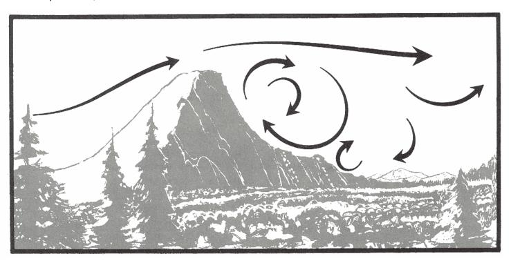
Large roll eddies are typical to the lee of bluffs or canyon rims. An upslope wind may be observed at the surface on the lee side.
