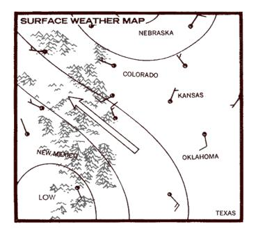
The wind direction at surface stations may differ widely from the windflow above the friction layer, as shown by this weather map. Surface wind direction is indicated on weather maps by a wind arrow flying with the wind. The number of barbs on the tail represent the wind speed. At the top of the friction layer the wind blows parallel to the isobars, as shown by the large arrow.
