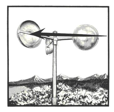
Horizontal wind speed is measured by the rate of rotation of a cup anemoter.
