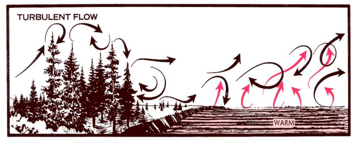
Roughness creates mechanical turbulence, while surface heating causes thermal turbulence in the airflow.
