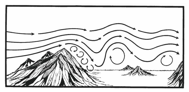
Mountain waves form when strong winds blow perpendicular to mountain ranges. Considerable turbulence and strong updrafts and downdrafts are found on the lee side. Crests of waves may be marked by lens-shaped wave clouds, but at times there may be insufficient moisture to form clouds.
