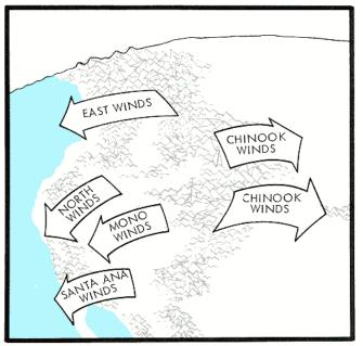
Foehn winds are known by different names in different parts of the mountains West. In each case, air is flowing from a highpressure area on the windward side of the mountains to a lowpressure area on the leeward side.
