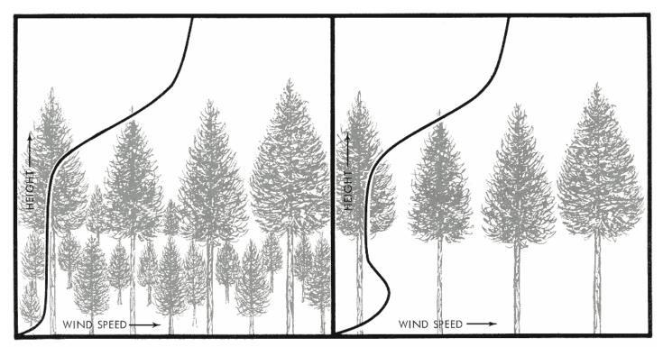
Vertical wind profiles in forest stands that the crown canopy is very effective in slowing down wind movement. In stands with an understory, the wind speed is nearly constant from just above the surface to near the tops of the crowns. Above the crowns, winds peed increases much like above level ground. In stands with an open trunk space, a maximum in wind speed is likely in the trunk space and a minimum in the crown area.
