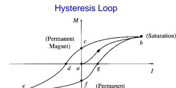
**Hysteresis**: The path we have traced out. In the experiment, we adjust the current *I*, i.e. control **H**. In practice *M* is huge compared to *H*.
