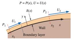
Outer flow speed parallel to the wall is U(x) and is obtained from the outer flow pressure, P(x). This speed appears in the *x*-component of the boundary layer momentum equation
