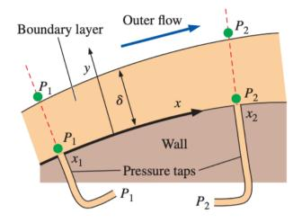
The pressure in the irrotational region of flow outside of a boundary layer can be measured by static pressure taps in the surface of the wall. Two such pressure taps are sketched. The pressure at the outer edge of a boundary layer can be measured experimentally by a static pressure tap at the wall directly beneath the boundary layer
