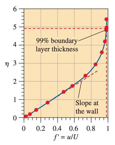
The Blasius profile in similarity variables for the boundary layer growing on a semi-infinite flat plate. Experimental data (show as circles) are at  $Re = 3.64 \times 10^5$ .
