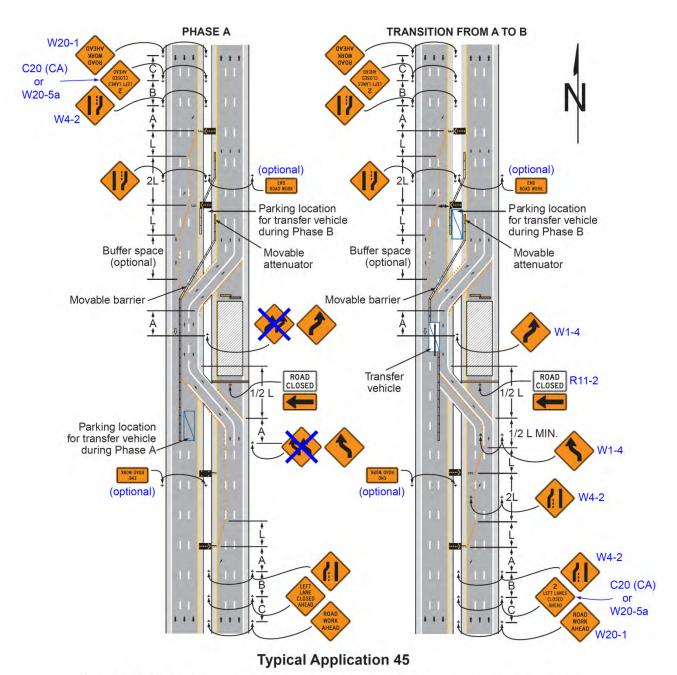
Note: See Tables 6H-2 and 6H-3 for the meaning of the symbols and/or letter codes used in this figure. Although leader lines point to the signs on the right-hand side of the roadway, most of these signs should be installed on both sides of the roadway.
