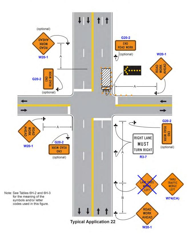
Figure 6H-22A(CA). Right-Hand Lane Closure on the Far Side of an Intersection (TA-22A (CA))
