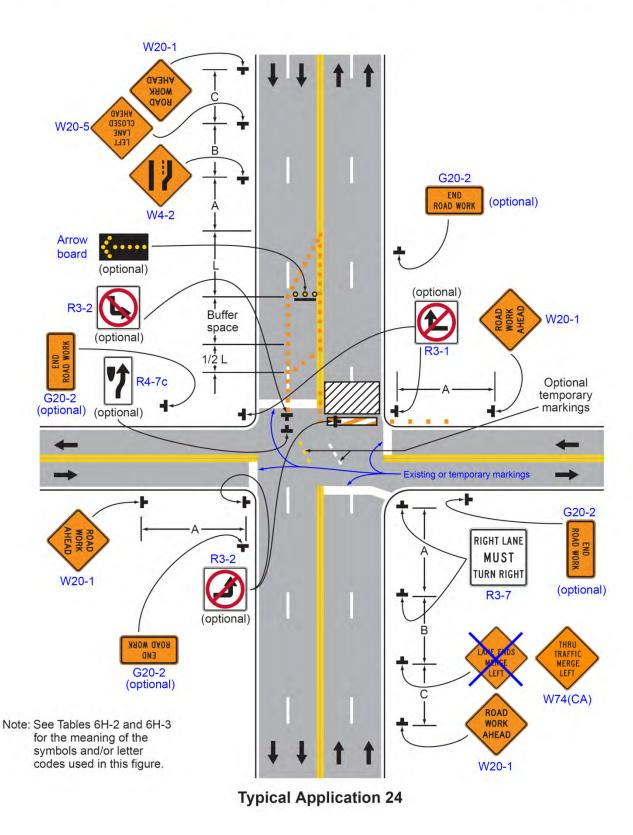
Figure 6H-24A (CA). Half Road Closure on the Far Side of an Intersection (TA-24A(CA))
