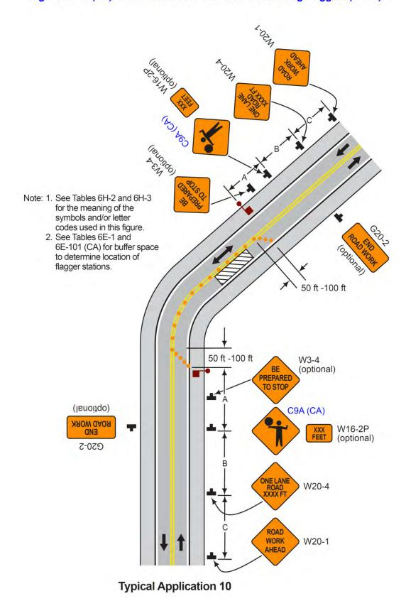
Figure 6H-10A (CA). Lane Closure on Two-Lane Road Using Flaggers (TA-10A)
