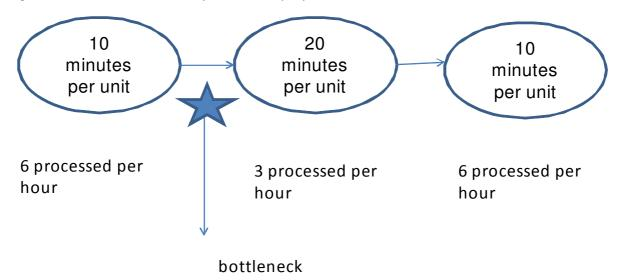
The diagram shows that the output of a process will be constrained by the slowest point. This is referred to as a 'bottleneck' in the process.
