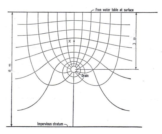
Figure 7.11. Flownet around the Horizontal Drain for Ex. 7.3
