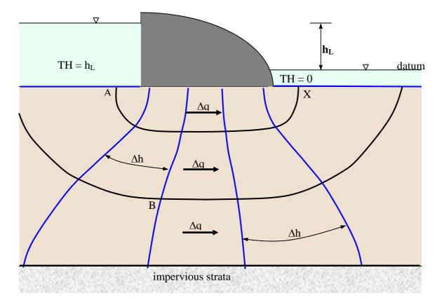
Figure 7.9 Streamlines and equipotential lines
