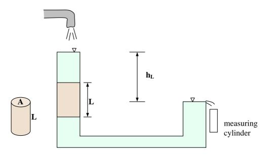
Figure 7.6 Constant head permeability test
