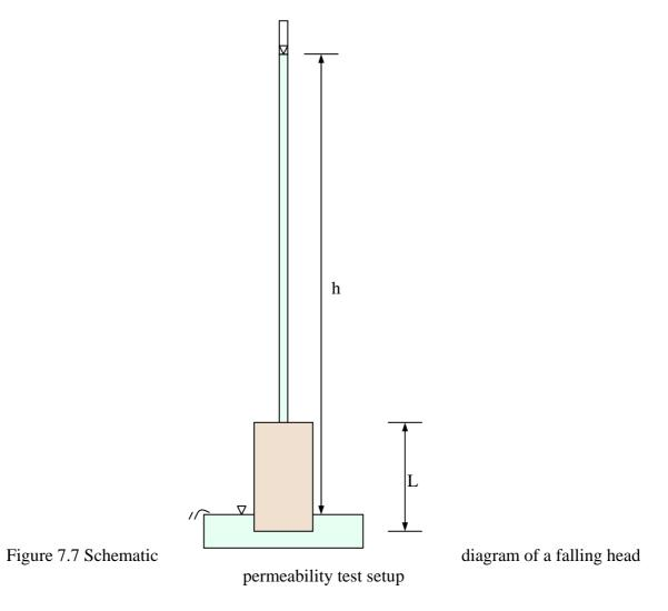
By applying Darcy's law, and equating the flow rate in the standpipe and the soil specimen, it can be shown that the permeability can be computed from Eq. 7.8
