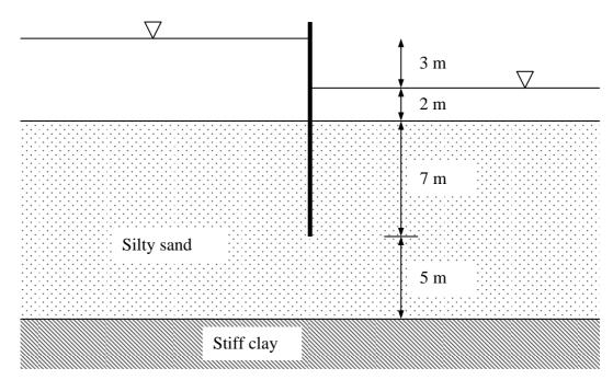
A stiff clay layer underlies a 12 m thick silty sand deposit. A sheet pile is driven into the sand to a depth of 7 m, and the upstream and downstream water levels are as shown in the figure. Permeability of the silty sand is  $8.6 \times 10^{-4}$  cm/s The stiff clay can be assumed to be impervious. The void ratio of the silty sand is 0.72 and the specific gravity of the grains is 2.65.
