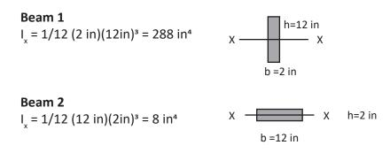
Under the same loading conditions, Beam 2 will bend before Beam 1.
