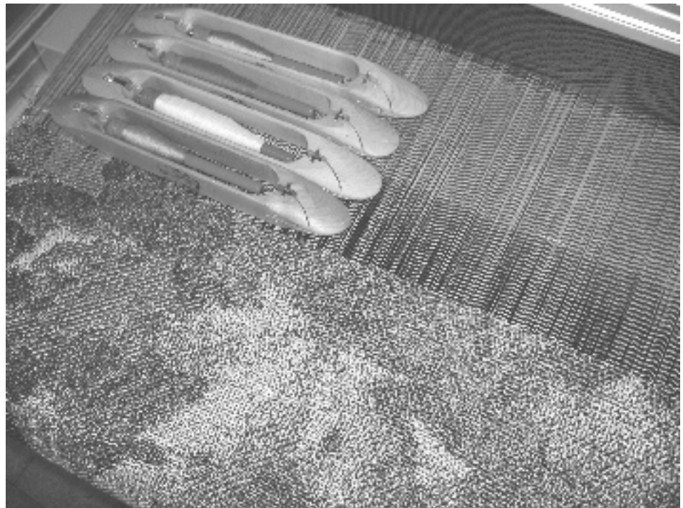
“Forest Floor” in progress: the structure is double twill with a four-color weft rotation. These weave presets may be found in the set DTwill4Wefts.pat.
