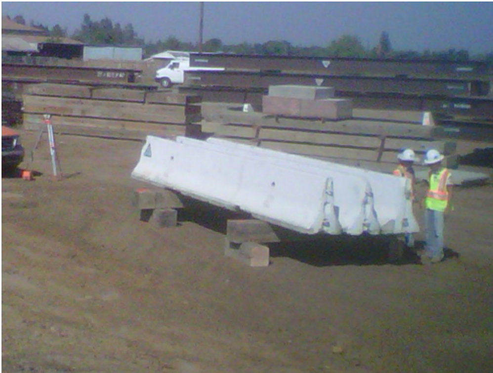
Figure 8-16. Simple Static Soil Load Test Using K-Rail.
