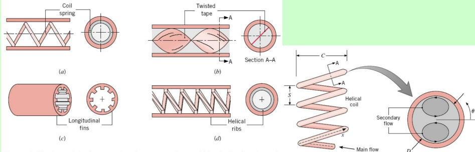
**FIGURE 8.12** Internal flow heat transfer enhancement schemes: (*a*) longitudinal section and end view of coil-spring wire insert, (*b*) longitudinal section and cross-sectional view of twisted tape insert, (*c*) cut-away section and end view of longitudinal fins, and (*d*) longitudinal section and end view of helical ribs.
