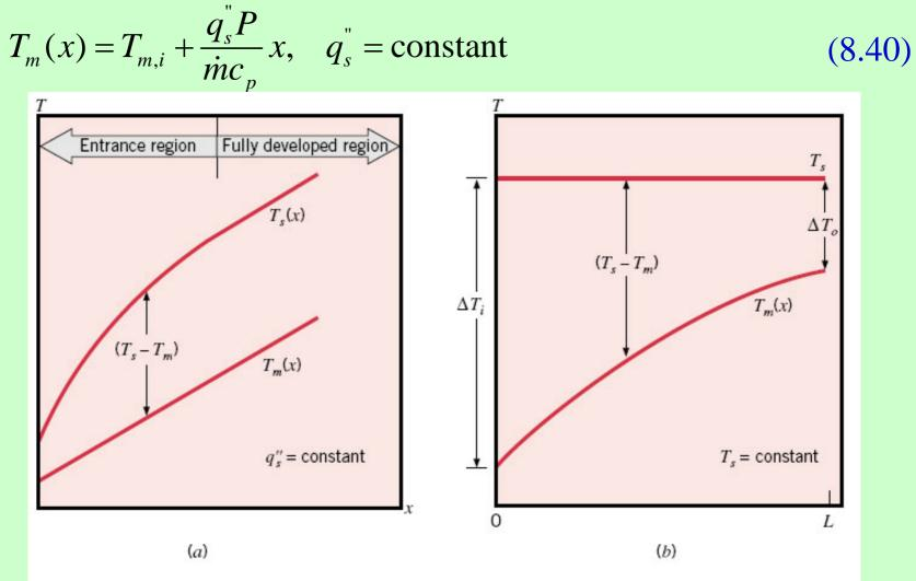
**FIGURE 8.7** Axial temperature variations for heat transfer in a tube. (*a*) Constant surface heat flux. (*b*) Constant surface temperature.
