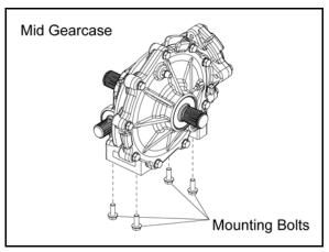
6. Slide the mid gearcase forward. Lift up on the gearcase to clear the frame and slide the gearcase towards the rear of the vehicle to remove the mid propshaft from the transmission.
