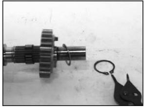
27. Remove bearing and the helical gear.
