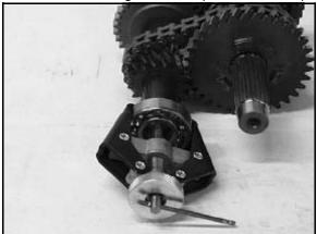
18. Remove the snap ring and washer from the reverse shaft.
