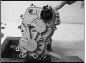
10. Lift shift rail 0.5"-1" (12.70-25.40 mm). Then rotate the shift rail / forks and shift drum, so the fork pins disengage from the drum.
