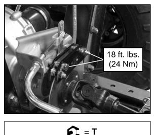
Parking Brake Caliper - Mounting Bolts: 18 ft. Ibs. (24 Nm)
