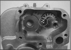
NOTE: Depending on what gear the transmission is in upon disassembly, the stamped timing marks may not be lined up. To avoid confusion, mark the two gears as described in Step 8.
