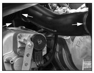
8. Disconnect the transmission switch and remove the pin clip from the shift cable end. Remove the washer and shift cable from the bellcrank.
