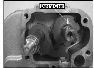
6. Mark the lockout disc, this will indicate which side of the disc faces outward during assembly. Remove the disc.
