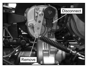
9. Loosen the transmission shift cable jam nuts. Remove the cable from the mounting bracket.
