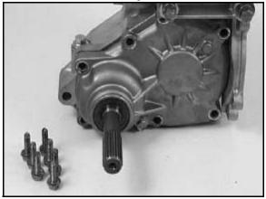
30. Remove the front housing cover, shim, thrust button, and thrust button shim.
