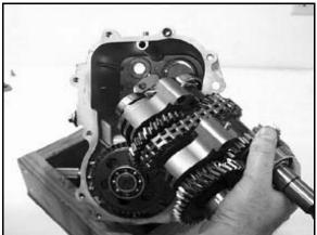
13. Set the upper gear cluster on a flat surface and inspect the components.
