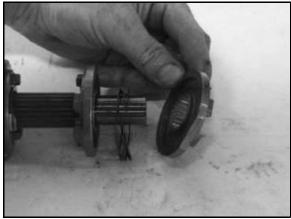
26. Remove the snap ring, washer, gear, and split bearing.
