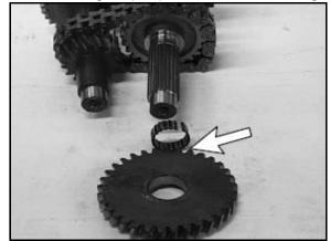
20. Remove the reverse gear shaft.
