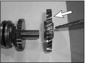
24. Remove the gear, split bearing, and washer from the reverse shaft.
