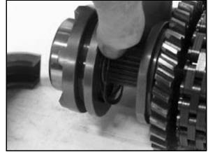
15. As the engagement dogs are installed onto the shaft, place the wave springs into the spring groove. Keep the spring in place while the fork is being installed on the shaft and while placing the shafts into the case.
