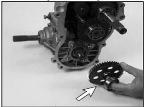
28. Remove the pinion shaft retainer plate and the pinion shaft.
