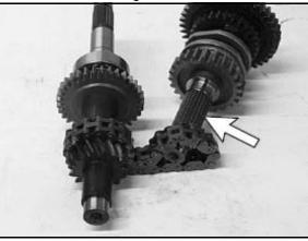
21. Remove the rest of the bearings from the shafts.
