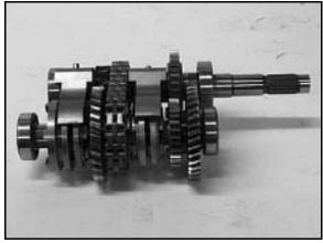
14. Remove the shift forks from the assembly. Note the correct position of each fork.
