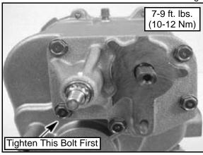
32. Torque the remaining cover bolts to specification.
