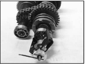
16. Remove the engagement dog. Remove the wave spring and reverse engagement dog.
