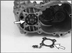
29. Remove the front housing cover screws.
