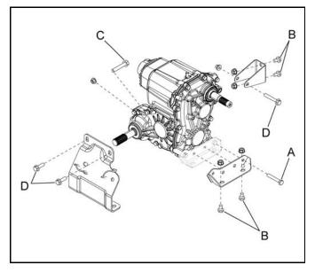
Transmission Mounting Bolts: B, C, D 40 ft. Ibs. (54 Nm)
