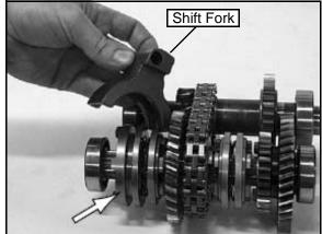
NOTE: The picture above depicts a transmission with a "Park" engagement dog on the end of the shaft instead of a regular engagement dog. The transmission will have a regular engagement dog in the location indicated by the arrow in the photo. 15. Remove the bearing from the reverse shaft with a puller.
