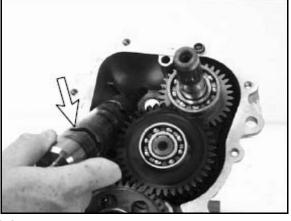
12. Remove the upper gear cluster and shift forks. You may need to move the assembly back and forth to aid in removal
