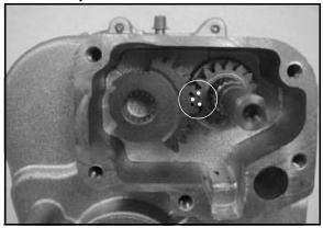
IMPORTANT: Note the location of the skip tooth on the splines. Apply a light coating of grease on the gear teeth.
