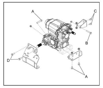
14. Remove transmission from right side of frame.
