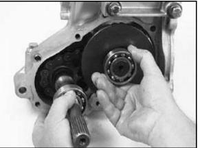
3. Before installing the cover make sure the sealing surfaces are clean and dry, and shafts are fully seated in the transmission case. Apply Polaris Crankcase Sealant to the mating surfaces.
