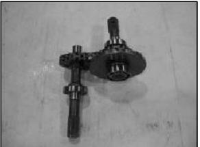
2. Install front and rear output shafts into the case.
