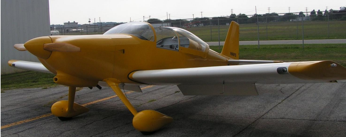
Figure 9.12. RV-6, N96FS, with the landing gear fairings ( http://picasaweb.google.com/lh/photo/1WDAfQ8oTdcM1tuSqvQ47A )
