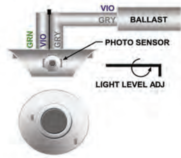
Figure 9.12.3. Photosensor and fluorescent dimming ballast for continuous daylight dimming.
