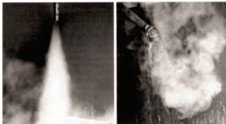
Figure 9.3.7. Live steam (left) versus flash steam (right)
