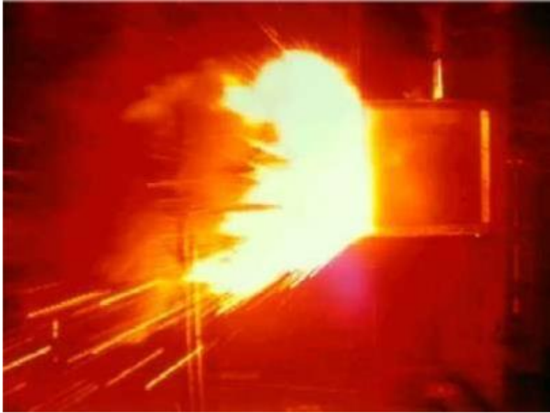
Fig. 9-31 Arc Flash Explosion
