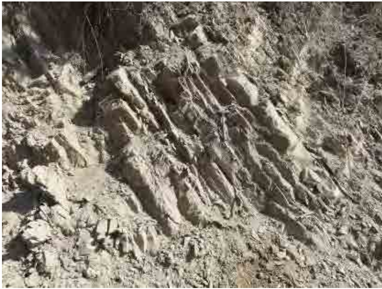
FIGURE 9.1-7 FEATURES OF BEDROCK WITH MANY CRACK
