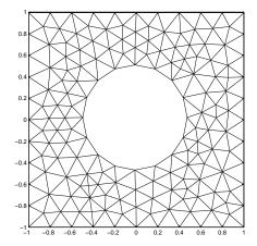
Figure 9.11. A mesh generated from Matlab.
