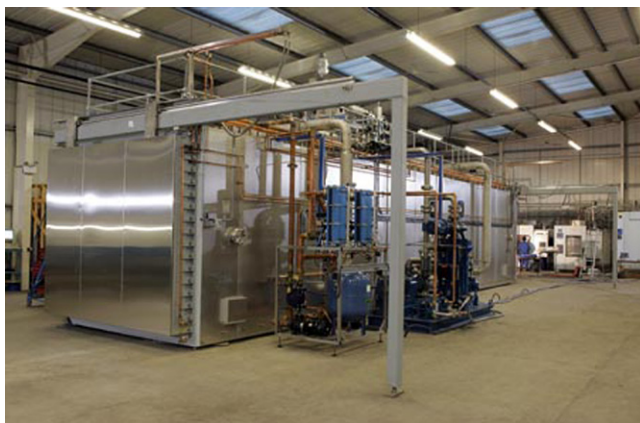
FIGURE III.1.2.5 Medium volume ethylene oxide production sterilization chamber manufactured by Getinge (Courtesy of Getinge Inc.).
