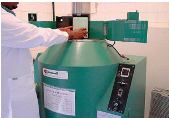
FIGURE III.1.2.3 Low volume self-contained R&D gamma cell manufactured by MDS Nordion (courtesy of IAEA, STI/PUB/1313).
