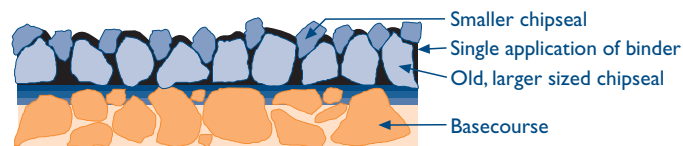
Figure 3-14 A voidfill seal (a single application of binder and small chip over existing seal).
