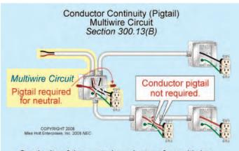
Continuity of the neutral conductor of a multiwire branch circuit must not be interrupted by the removal of a wiring device.
