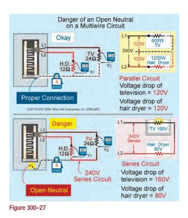
**WARNING:** Failure to terminate the ungrounded conductors to separate phases can cause the neutral conductor to become overloaded, and the insulation can be damaged or destroyed by excessive heat. Conductor overheating is known to decrease the service life of insulating materials, which creates the potential for arcing faults in hidden locations, and could ultimately lead to fires. It isn't known just how long conductor insulation lasts, but heat does decrease its life span. Figure 300–28
