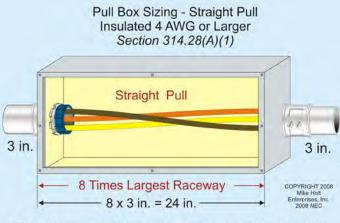
The distance from the conductors' entry to the opposite wall must not be less than 8 times the largest raceway.
