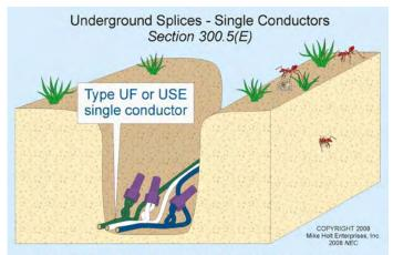
Single Type UF or USE conductors can be spliced underground with a device that is listed for direct burial.
