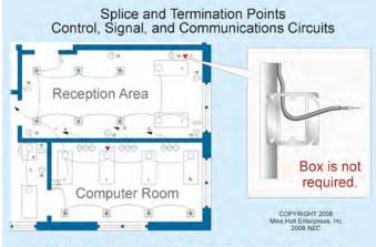
A box is not required for communications, signal, and control conductors [90.3, 725.3, and 770.3].
