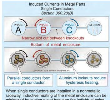
minimized by cutting a slot between the individual holes through which the conductors pass.
