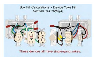
Each device yoke counts as two conductors, based on the largest conductor terminating on the device.
