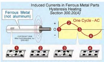
Ferrous metal (steel and iron) molecules align to the polarity of the magnetic field, and when the field reverses, the molecules reverse their polarity. This back-and-forth alignment of the molecules heats up ferrous metal parts.
