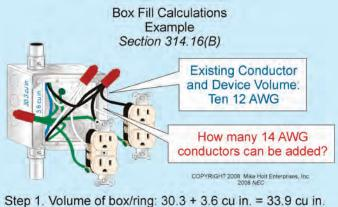
Step 1. Volume of boxring: 30.3 + 3.6 cu in. = 33.9 cu in. Step 2. Volume of existing conductors/devices = 22.5 cu in. Step 3. Space remaining: 33.9 - 22.5 = 11.4 cu in. Step 4. Number of 14 AWG added: 11.4/2.0 cu in. = 5
