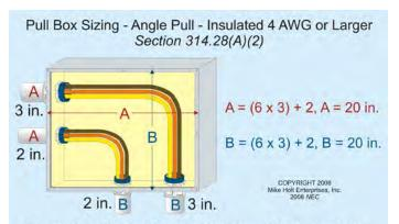
For angle pulls, the distance (measured from conductor wall entry to the opposite wall) must not be less than 6 times the largest raceway, plus the sum of the diameters of the remaining raceways on the same wall and row.
