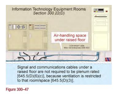
**Author's Comment:** Signal and communications cables under a raised floor are not required to be suitable for plenum use [645.5(D)(6)(c)], because ventilation is restricted to that room/ space, and the space is not normally occupied [645.5(D)(4)].
