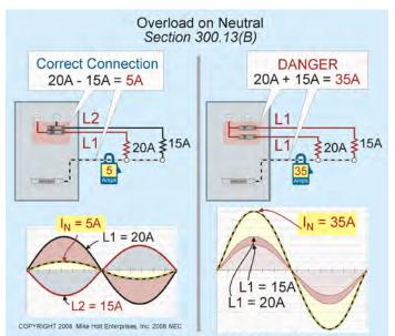
Failure to terminate the ungrounded conductors to different phases or lines can cause the neutral conductor to be overloaded, which can cause a fire.
