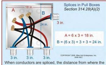
when conductors are spliced, the distance from where the raceways enter to the opposite wall must not be less than six times the largest raceway plus the sum of all other raceways on the same wall and row.
