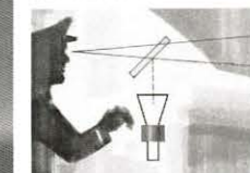
Is visible to pilot through half-silvered mirror...
