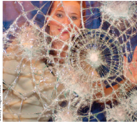
Figure 14-20. Fracture patterns on tempered glass.
