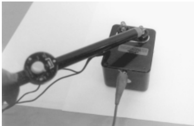
Figure 7-15 Using a high voltage tester to check an ignition transformer. Each terminal should read 5,000 volts.
