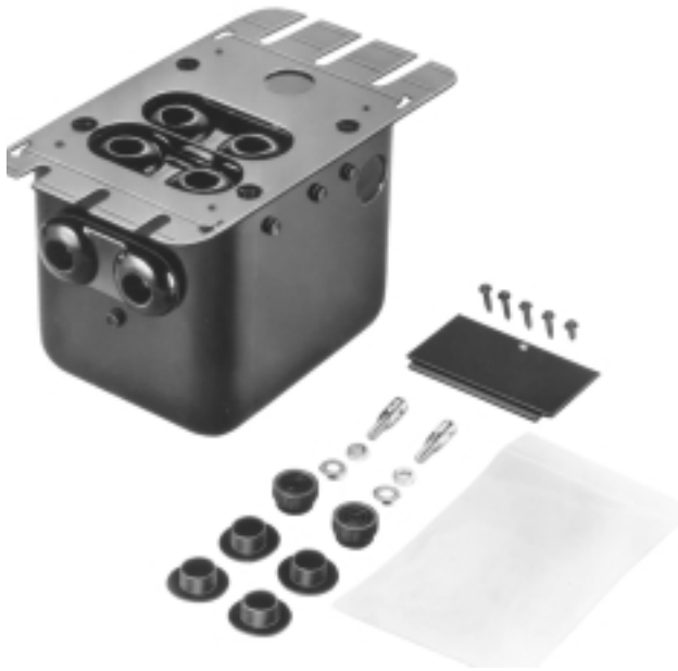
Figure 7-6 Universal replacement ignition transformer can be adapted to fit a variety of oil burners and reduces the stock inventory of the service vehicle. Courtesy: Webster Heating Products, Inc.
