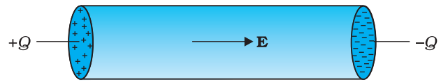
FIGURE 3.1 Charges +Q and -Q put at the ends of a metallic cylinder. The electrons will drift because of the electric field created to neutralise the charges. The current thus will stop after a while unless the charges +Q and -Q are continuously replenished.
