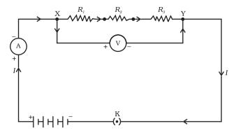
Figure 12.6 Resistors in series
