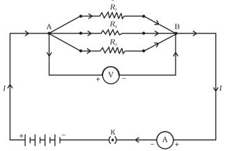
Figure 12.7 Resistors in parallel
