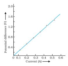
**Figure 12.3**V-I graph for a nichrome wire. A straight line plot shows that as the current through a wire increases, the potential difference across the wire
