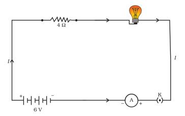
**Figure 12.9** An electric lamp connected in series with a resistor of  $4 \Omega$  to a 6 V battery
