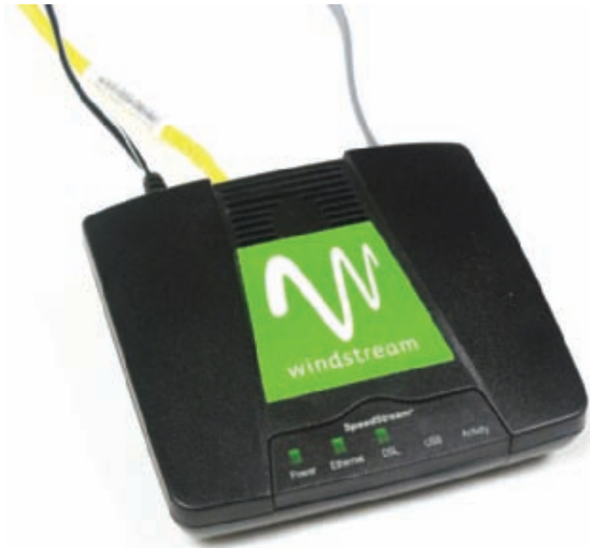
Figure 17-4 This DSL box connects to a phone jack and a PC to provide a broadband connection to an ISP Courtesy: Course Technology/Cengage Learning
