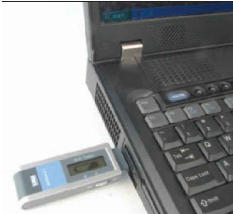
Figure 17-60 Plug the wireless USB adapter into the USB port Courtesy: Course Technology/Cengage Learning
