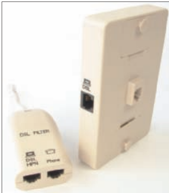
Figure 17-2 When DSL is used in your home, filters are needed on every phone jack except the one used by the DSL modem Courtesy: Course Technology/Cengage Learning
