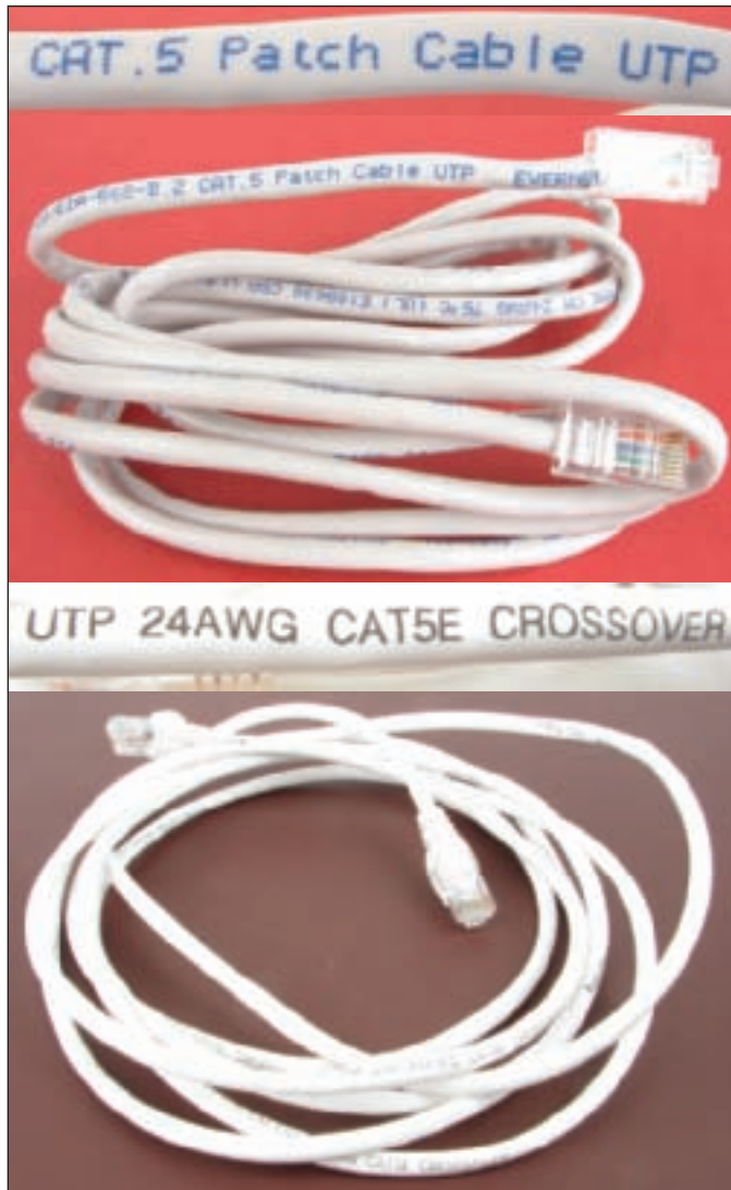
Figure 17-25 Patch cables and crossover cables look the same but are labeled differently Courtesy: Course Technology/Cengage Learning
