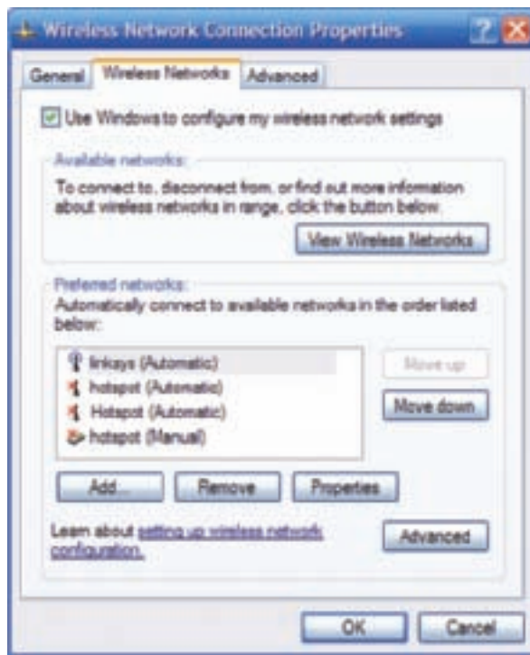
Figure 17-74 Manage wireless hot spots using the Wireless Network Connection Properties box Courtesy: Course Technology/Cengage Learning
