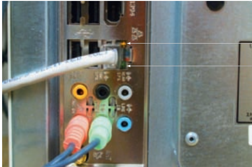
Figure 17-15 Status indicator lights for the embedded network port Courtesy: Course Technology/Cengage Learning
