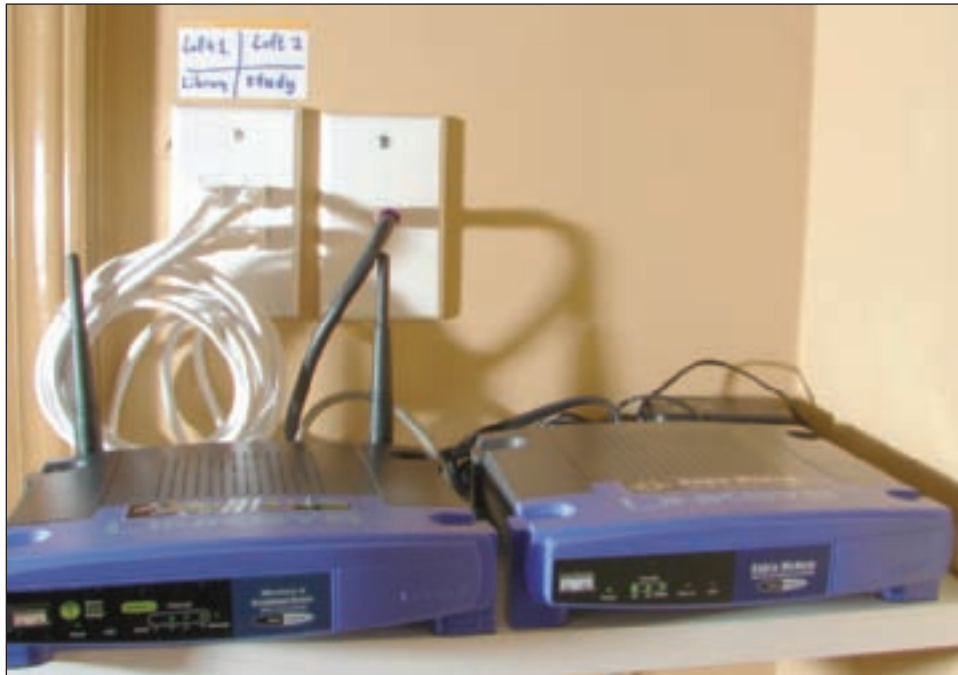
Figure 17-30 A router and cable modem are used to provide Internet access for a small network Courtesy: Course Technology/Cengage Learning
