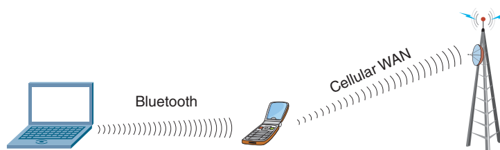
Figure 17-10 Bluetooth can be used for short transmissions between personal devices such as a cell phone and notebook computer. Courtesy: Course Technology/Cengage Learning
