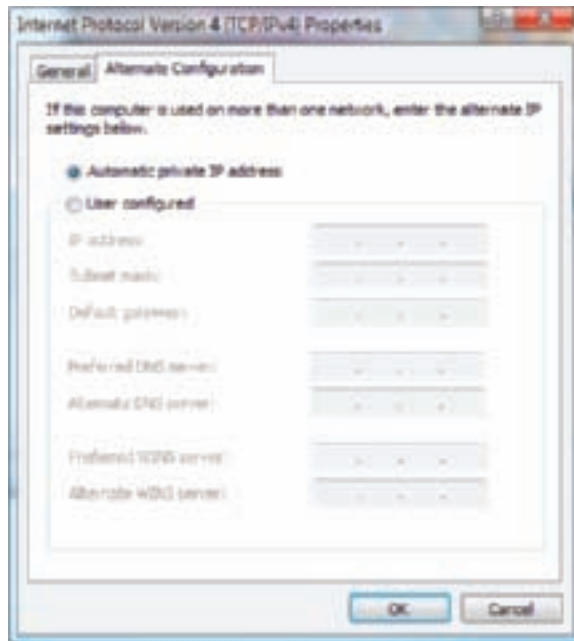
Figure 17-59 Alternate configuration that applies if the first TCP/IP settings do not work Courtesy: Course Technology/Cengage Learning
