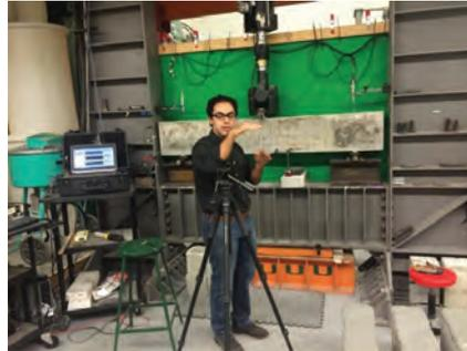
PhD student Houman Akbari Hadid shows the fatigue testing they are doing on a control beam sample
