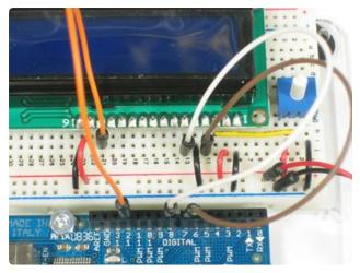
Now we will wire up the data pins. DB7 is pin #14 on the LCD, and it connects with an orange wire to Arduino #12.
