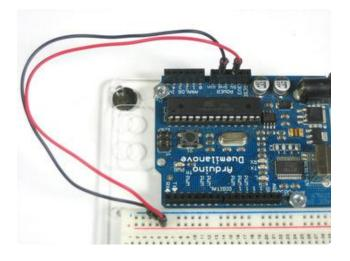
Now we'll provide power to the breadboard. Connect +5V to the red rail, and Ground to the blue rail.
