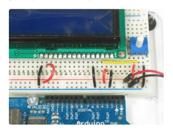
As mentioned, we'll not be using the RW pin, so we can tie it go ground. That's pin 5 as shown here.
