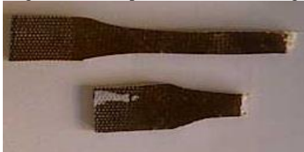
Figure 2.6: Tensile specimen after testing
