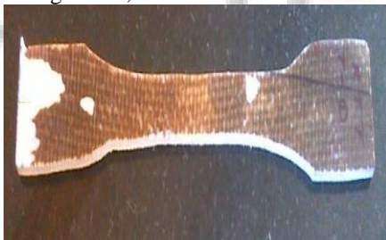
Fig.2.5 Tensile specimen before testing
