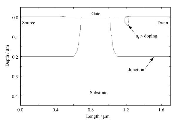
Fig. 3.38 A contour within which the intrinsic carrier concentration,  $n_i$ , is greater than the background doping level is drawn for a simulation structure at the time of peak ESD stress. Lines are also drawn marking the source and drain junctions of the structure, which is not plotted to scale.
