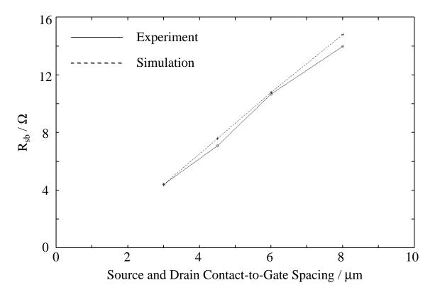
Fig. 4.45 Experimental and simulated snapback resistance,  $R_{sb}$ , vs. contact-to-gate spacing for a 50/0.75 $\mu$ m MOSFET test structure. The contact-to-gate spacing refers to the distance from the drain contacts to the gate edge and the source contacts to the gate edge.
