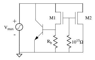
Fig. 3.28 ESD protection circuit used for SPICE simulations by Chatterjee et al. [33]. M1 is an NMOS transistor designed to facilitate the turn-on of the npn transistor during ESD. M2 represents the output NMOS transistor being protected.
