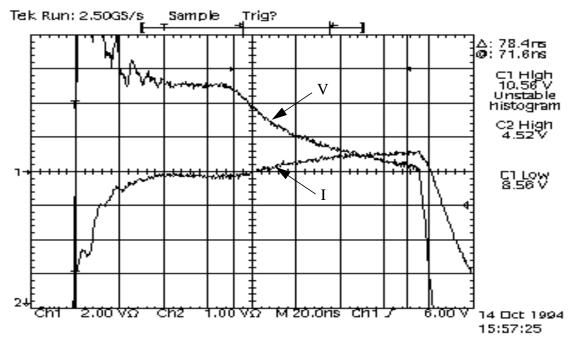
Fig. 2.10 Second breakdown is observed as a drop in the device voltage and rise in device current about 72ns into the 36V, 150ns input pulse.
