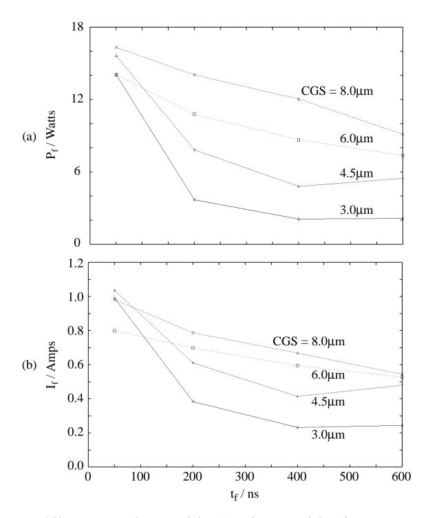
Fig. 4.53 Experimental power-to-failure (a) and current-to-failure (b) vs. time-to-failure,  $t_f$  for 50/0.75µm test structures with varying contact-to-gate spacings (CGS). In these plots, the time to failure is equal to the TLP pulse width and the failure condition is defined as 1µA leakage.
