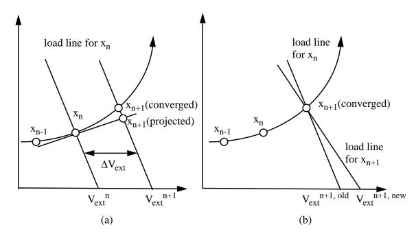
Fig. 3.25 (a) Projection: the solution is advanced by incrementing the external voltage from  $V_{\rm ext}^{\ \ n+1}$  while the load resistance is held constant; (b) Recalibration: the load resistance is changed so that the load line is perpendicular to the trace at the new solution point. This implies a new external voltage ( $V_{\rm ext}^{\ \ n+1, new}$ ).
