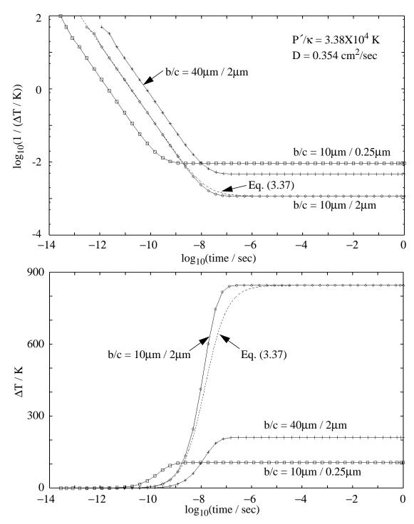
Fig. 3.32 Simulated  $1/\Delta T$  vs. time (a) and  $\Delta T$  vs. time (b) curves for various length/width ratios in a uniformly doped semiconductor region with a constant applied power. The temperature on the perimeter of the rectangular device is fixed at 300K. Eq. (3.37), the analytic approximation, is plotted for the  $10\mu m$  X  $2\mu m$  structure.
