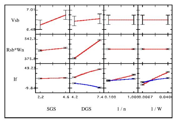
Fig. 5.60 Catalyst model graph for Lot 1  $V_{sb}$ ,  $R_{sb}$  (multiplied by structure width), and normalized  $I_{TLP,ws}$  (If) as a function of SGS, DGS, 1/n, and 1/W.
