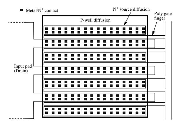
Fig. 2.19 Layout of a multiple-finger NMOS transistor between input and  $V_{SS}$ . There are three drain fingers and six poly gates. Another finger (not shown) branches off of the drain pad to the input buffer of the IC.
