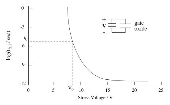
Fig. 3.35 A qualitative plot of time-to-failure vs. stress voltage reveals the time-dependent dielectric breakdown behavior of a gate oxide. If the voltage  $V_0$  is applied across the oxide for a time greater than  $t_0$ , the oxide will rupture.
