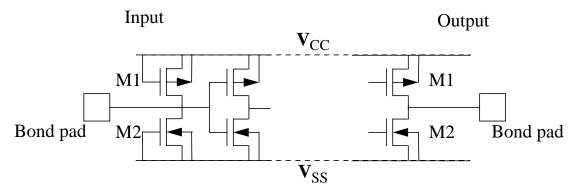
Fig. 2.16 CMOS input and output protection. The input protection transistors protect the thin gates of the input buffer, while the output protection transistors double as the output buffer.
