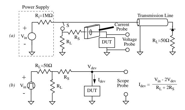
Fig. 2.14 (a) Advanced TLP schematic: a series-parallel resistor combination has been added to enhance current resolution. A current probe is now used to directly measure the device current on the oscilloscope. (b) Equivalent circuit of the TLP setup.
