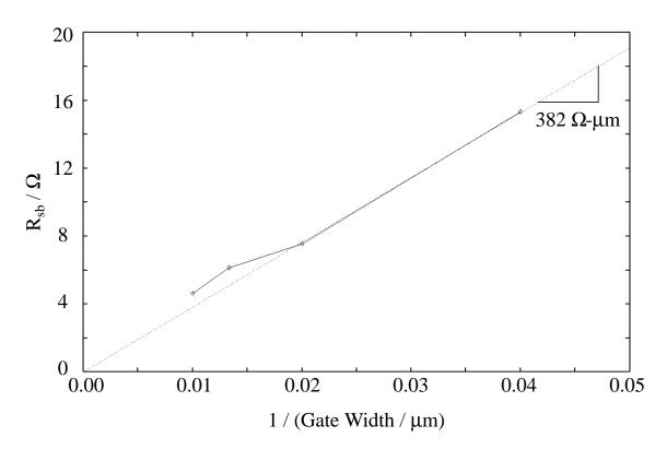
Fig. 4.46 Experimental snapback resistance,  $R_{sb}$ , (connected points) vs. inverse gate width, W, for 0.75 $\mu$ m test structures. The dashed line indicates that  $R_{sb} \times W = 382\Omega$ - $\mu$ m for gate widths less than 50 $\mu$ m.
