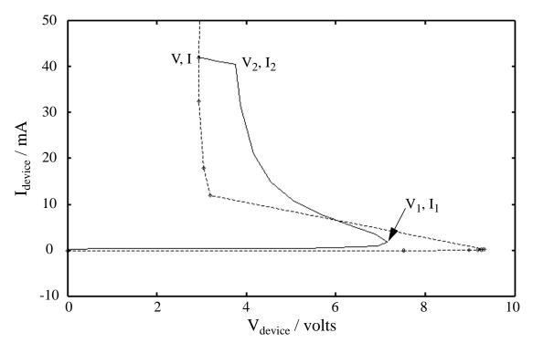
Fig. 3.30 I-V curves of a single TLP simulation (solid line,  $V_{\rm in}$ =50V in the circuit of Fig. 3.27) and of points resulting from a group of TLP simulations (dashed line). Point ( $V_1$ ,  $I_1$ ) corresponds to the turn-on of the parasitic bipolar transistor.  $V_2$  and  $I_2$  are the device voltage and current values at the time the input pulse reaches its peak; in this case  $t_{\rm rise} = 1$ ns. The quasi-steady state of the pulse is the point ( $V_1$ ).
