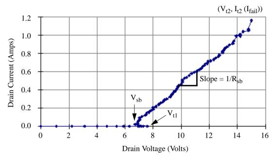
Fig. 5.54 Snapback I-V curve for a 50/0.6 $\mu$ m NMOS transistor generated by TLP. Critical I-V parameters are the trigger voltage ( $V_{t1}$ ), snapback voltage ( $V_{sb}$ ), snapback resistance ( $R_{sb}$ ), and thermal-runaway or second-breakdown point ( $V_{t2}$ ,  $I_{t2}$  ( $I_{fail}$ )).
