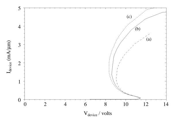
Fig. 4.43 Simulated I-V sweep for T=297K boundary conditions on (a) electrical contacts; (b) perimeter of simulation structure; and (c) perimeter of structure with reduced dependence of impact-ionization rate on temperature.
