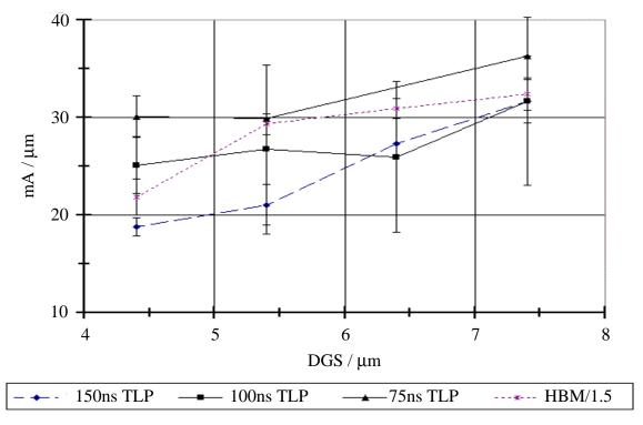
Fig. 5.56 Normalized (divided by width) withstand current vs. drain-side CGS for HBM stressing and 75, 100, and 150ns TLP stressing of 50/0.6µm single-finger transistors. For HBM, the withstand voltage is converted to mA by dividing by 1.5. Error bars represent 95% confidence intervals.
