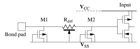
Fig. 2.18 Combination resistor/transistor ESD input protection circuit, featuring a diffused resistor (R<sub>diff</sub>) between wide (M1) and narrow (M2) NMOS transistors. Resistance from gate to ground is not shown.
