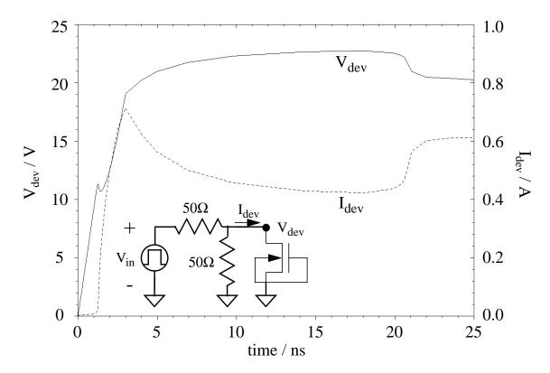
Fig. 4.44 Device voltage and current vs. time for a transient simulation of the 100/0.75µm structure (cf. Fig. 2.10). Second breakdown is observed at 21ns, corresponding to a peak temperature in the device of 1510K. The simulation circuit is shown inset.
