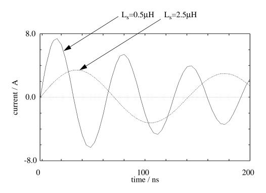
Fig. 2.3 SPICE-generated short-circuit MM output current waveforms for  $V_c$ =400V,  $C_c$ =200pF,  $R_c$ =5 $\Omega$ ,  $C_s$ =1pF, and  $C_t$ =10pF.
