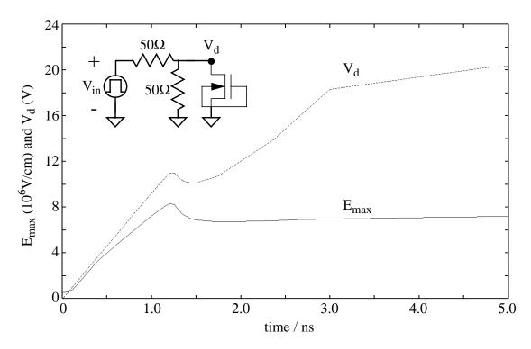
Fig. 3.34 The maximum electric field in the gate oxide ( $E_{max}$ , in MV/cm) of an ESD-protection MOSFET subjected to a square pulse with a 3ns rise time is plotted vs. time. As seen from the plot of the input voltage at the drain of the device,  $V_{d}$ , the reduction in  $E_{max}$  is due to the device snapping back at 1.2ns.
