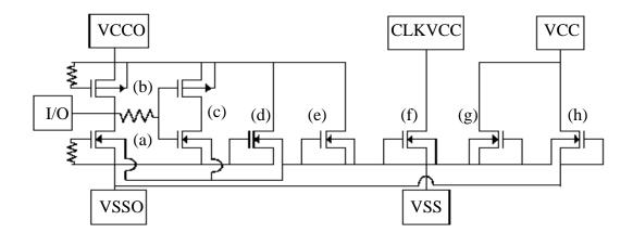
Fig. 5.59 Schematic of critical ESD protection circuits in a chip with split power supplies (VCCO/VSSO and VCC/VSS) and separate clock supply (CLKVCC): (a) n-channel pull-down, (b) p-channel pull-up, (c) CMOS pair representing internal circuitry, (d)-(h) n-channel clamps between various supplies (clamps for VCC-VCCO, VCC-CLKVCC, and VCCO-CLKVCC not shown).
