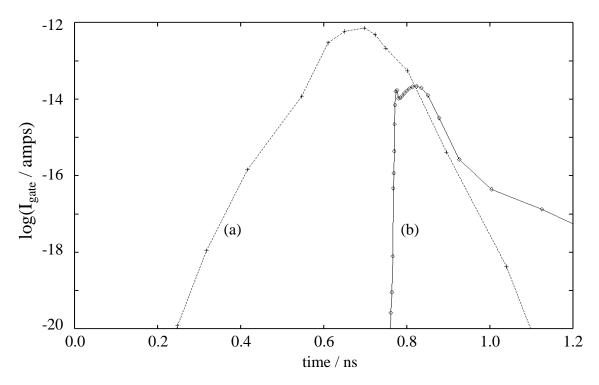
Fig. 3.36 Gate current vs. time for  $50/0.75\mu m$  MOSFETs with (a)  $10K\Omega$  gate resistor and (b) grounded gate. The drain is subjected to a square-wave pulse with a rise time of 3ns as depicted in the inset of Fig. 3.34. For both structures, the peak in gate current coincides with the time snapback occurs.
