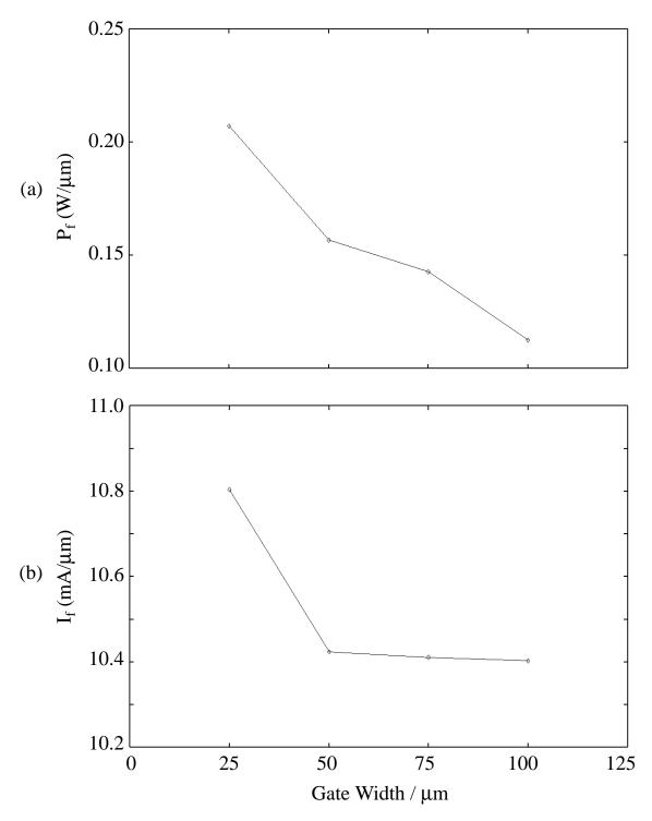
Fig. 4.49 Power to failure,  $P_f$  (a) and current to failure,  $I_f$  (b) vs. device width for 0.75 $\mu$ m test structures subjected to stepped 200ns transmission-line pulses. Each value is divided by the device width to normalize the results.
