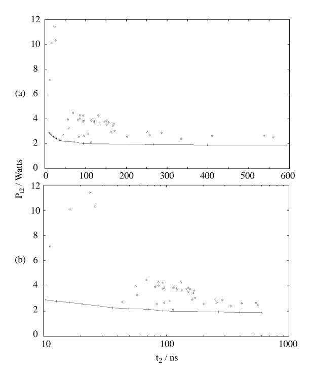
Fig. 4.52 Power at second breakdown,  $P_{t2}$ , vs. time to breakdown,  $t_2$ , for a  $25/0.75 \mu m$  structure plotted on linear (a) and semi-log (b) scales. Experimental results (points) are extracted from TLP experiments using various pulse lengths, while simulation points (line) are taken from simulations with varying pulse heights of indefinite width.
