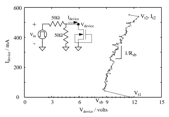
Fig. 4.41 I-V points from the transmission-line pulse sweep of a standard  $50/0.75 \mu m$  test structure (equivalent circuit shown inset). The trigger voltage  $(V_{t1})$ , snapback voltage  $(V_{sb})$ , snapback resistance  $(R_{sb})$ , and second-breakdown point  $(V_{t2}, I_{t2})$  can be extracted from the curve.
