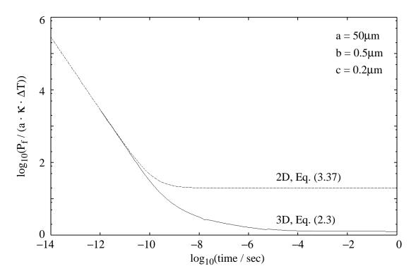
Fig. 3.33 Power to failure, normalized by a,  $\kappa$ , and  $\Delta T$ , is plotted vs. time to failure for the 2D and 3D implementations of the thermal box model. The time constants for the given box dimensions are  $t_a = 5.6 \mu s$ ,  $t_b = 560 ps$ , and  $t_c = 90 ps$ .
