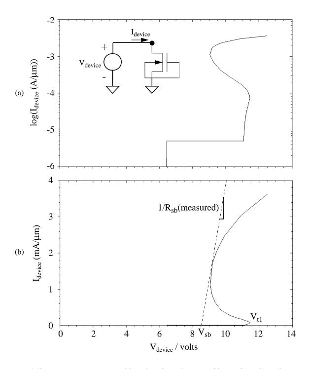
Fig. 4.42 Device current per width is plotted on a log (a) and linear (b) scale vs. device voltage for a dc-sweep simulation of the standard structure with proper gridding and impact-ionization modeling. The snapback voltage is extracted using a line determined by the measured snapback resistance. To compare the linear curve to Fig. 4.41, multiply the current per width by 50µm.
