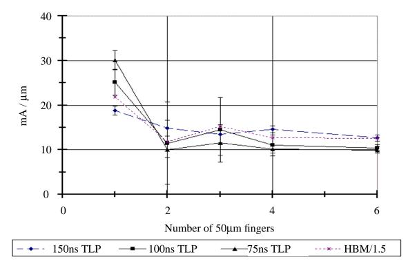
Fig. 5.57 Normalized (divided by width) withstand current vs. number of 50/0.6µm fingers for HBM stressing and 75, 100, and 150ns TLP stressing. Error bars represent 95% confidence intervals.
