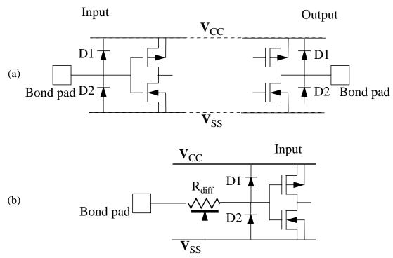
Fig. 2.15 (a) ESD diode protection circuit in a CMOS technology; (b) use of a series resistor in combination with diode protection. A diffused resistor has a distributed resistance and also forms a distributed diode.
