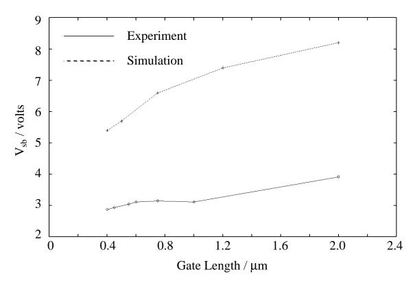
Fig. 4.47 Experimental and simulated snapback voltage,  $V_{sb}$ , vs. gate length for 20 $\mu$ m-wide test structures. The experimental results are for fully salicided structures, while the simulation results are for structures with 1.0 $\mu$ m CGS.
