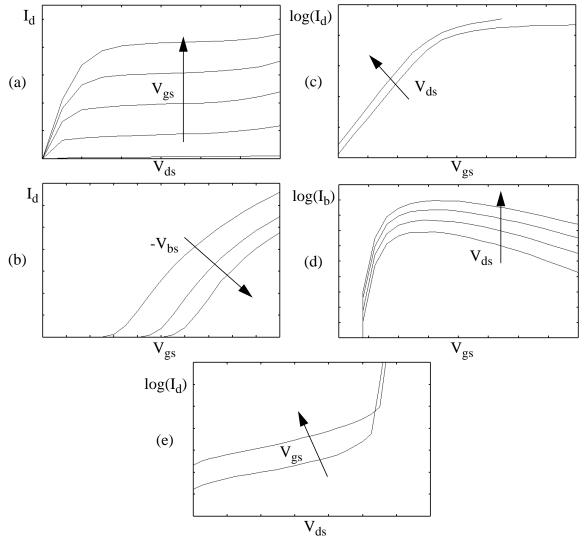
Fig. 4.40 Qualitative depiction of I-V curves used for MOSFET calibration: (a) drain:  $I_d$  vs.  $V_{ds}$  for stepped  $V_{gs}$ ; (b) gate:  $I_d$  vs.  $V_{gs}$  for stepped  $V_{bs}$ ; (c) subthreshold:  $log(I_d)$  vs.  $V_{gs}$  for stepped  $V_{ds}$ ; (d) substrate:  $log(I_b)$  vs.  $V_{gs}$  for stepped  $V_{ds}$ ; (e) breakdown:  $log(I_d)$  vs.  $V_{ds}$  for stepped  $V_{gs}$ . The subscripts d, s, g, and b refer to the drain, source, gate, and substrate, respectively.
