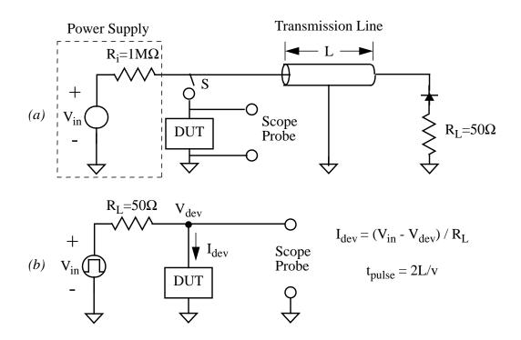
Fig. 2.5 (a) TLP schematic: a transmission line of length L is charged to voltage V<sub>in</sub> and then discharged through the device under test (DUT) when switch S closes. An oscilloscope voltage probe across the DUT monitors the circuit response. (b) Equivalent circuit of the TLP setup: the input is a square pulse of height V<sub>in</sub> and duration 2L/v, where v is the phase velocity of the line.
