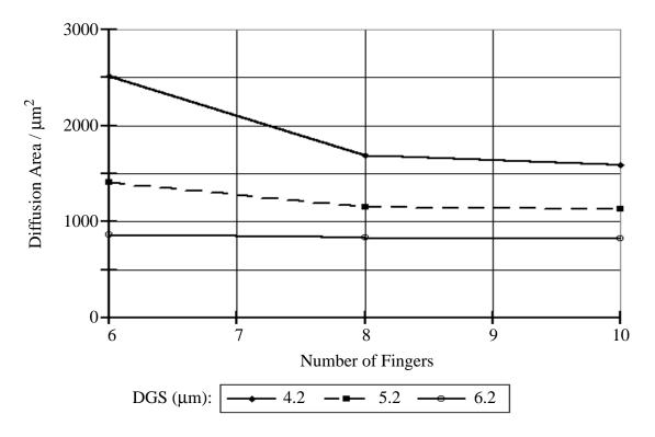
Fig. 5.61 Calculated minimum area of transistor source/drain diffusion needed for 5kV HBM protection for various DGS and number of fingers for Lot 1 with a SGS of 2.2µm.
