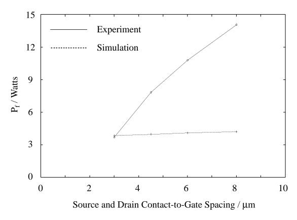
Fig. 4.50 Simulated and experimental power-to-failure,  $P_f$  vs. contact-to-gate spacing for 50/0.75 $\mu$ m test structures subjected to 200ns TLP pulses.
