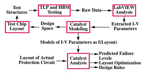
Fig. 5.62 Block diagram of ESD circuit design methodology.
