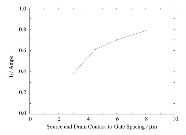
Fig. 4.51 Experimental current-to-failure,  $I_f$  vs. contact-to-gate spacing for  $50/0.75 \mu m$  test structures subjected to 200ns TLP pulses.
