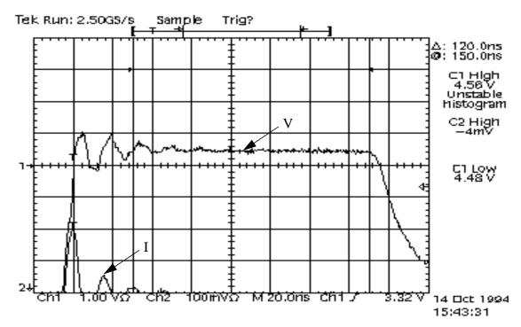
Fig. 2.8 A screen capture of a Tektronix TDS 684A digitizing oscilloscope displays the device voltage (Ch1) and current (Ch2) response of a 50/0.6µm device to a 4.6V, 150ns input pulse. After some initial ringing, the device voltage settles to a value approximately equal to the input voltage and the device current is very small. The current probe registers 5mV per 1mA of current.
