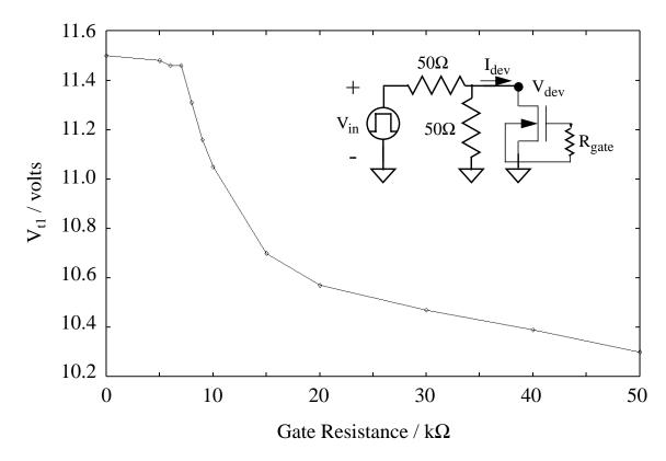
Fig. 4.48 Simulated trigger voltage,  $V_{tl}$ , vs. gate resistance,  $R_{gate}$ , for the 50/0.75 $\mu$ m test structure. Simulations predict that  $R_{gate}$  does not have a significant effect until it reaches a value of about  $10k\Omega$
