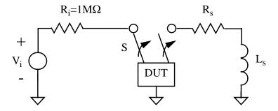
Fig. 2.4 Circuit model for the CDM. A ground pin of the device under test (DUT) is charged to a voltage V<sub>i</sub>, after which the switch S is thrown, removing the voltage source and connecting a different pin of the device to ground.
