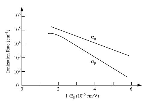
Fig. 3.22 Qualitative plot of impact-ionization rates for electrons  $(\alpha_n)$  and holes  $(\alpha_p)$  as a function of electric field for silicon at 300K.
