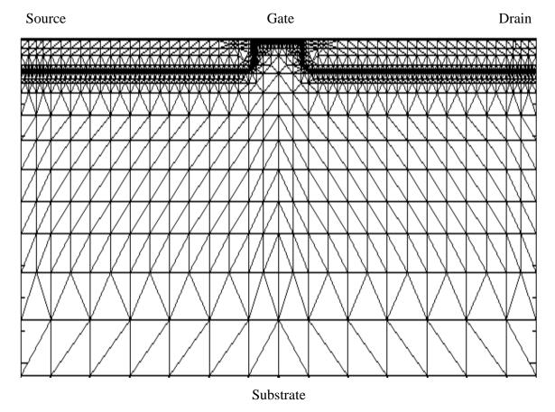
Fig. 4.39 This example of a MEDICI-generated grid shows the concentration of grid points in the channel, LDD, and junction regions. Several microns of the substrate portion of the simulated structure have been omitted in order to display the grid approximately to scale.
