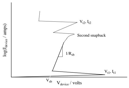
Fig. 2.7 Depiction of second snapback in a qualitative transient I-V curve for an NMOS transistor subjected to a positive ESD pulse.
