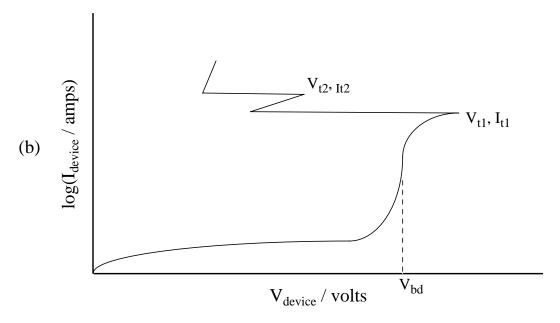
Fig. 2.6 Qualitative I-V curve for an NMOS transistor subjected to a positive ESD pulse: (a) linear scale shows snapback trigger point  $(V_{t1}, I_{t1})$ , snapback voltage  $(V_{sb})$  and resistance  $(R_{sb})$ , and second-breakdown trigger point  $(V_{t2}, I_{t2})$ , with circuit shown inset; (b) log scale shows the difference between device breakdown voltage  $(V_{bd})$  and snapback trigger point.
