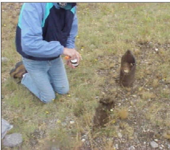
Figure 18. Sampling a 155-mm round that was broken open by a low-order detonation.
