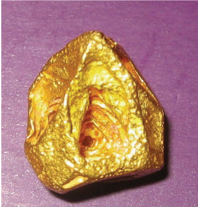
Figure 2. Gold crystal from Icabarú, Bolívar, Venezuela. It is also shown in the bottom right of figure 1. The front, hopped face is the one that produced the diffraction pattern in figure 8b.
