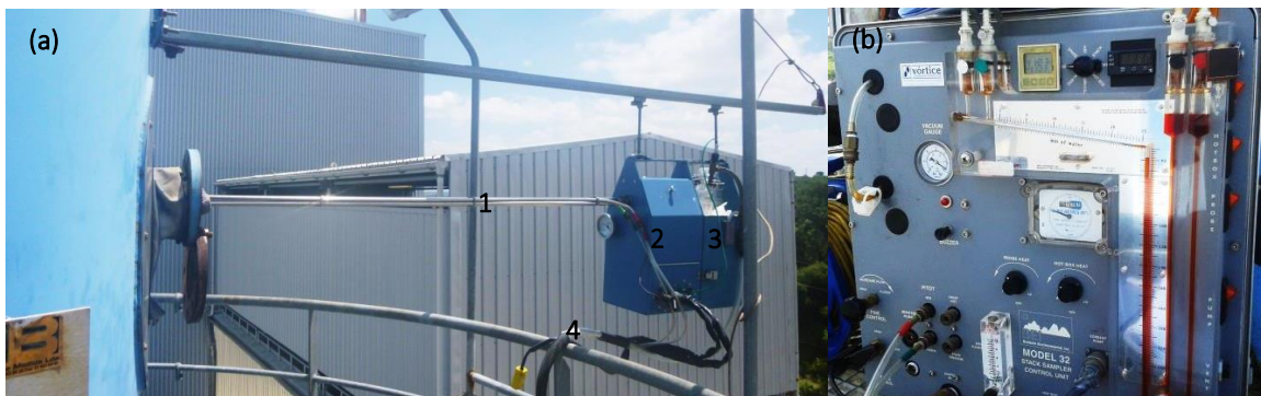
Figure 13 – Sampling train: (a) 1 Probe, 2 Heated area, 3 Ice bath, 4 Umbilical cord (b) Control Unit
