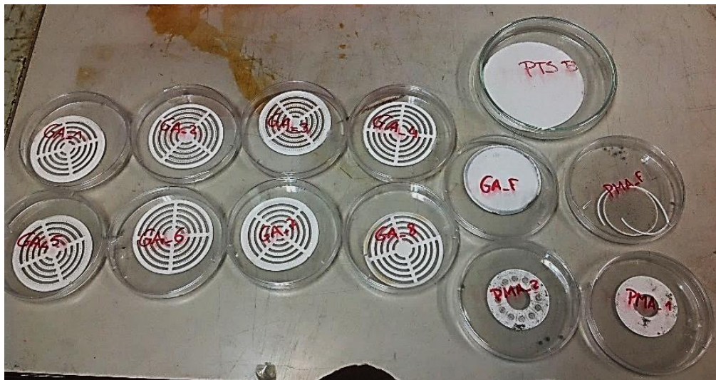
Figure 27 – Filters with particles of sampling GA (Mark III), PMA(TECORA MSS1) and TSPB (TSP)
