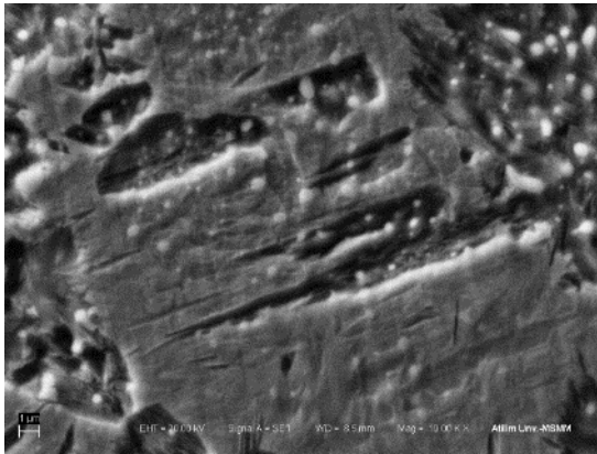
Figure 29: SEM Image of set No3.7 with t_{8/5} : 27 s. 10K X magnification. Martensitic and bainitic microstructure.
