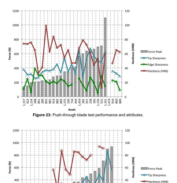
The weapons with low peak forces tend to exhibit higher tip sharpness values (lower force) for both the blades and spikes. Edge sharpness for the blades did not correspond to peak force. Material hardness readings for the blades and spikes presented in the figures vary considerably and may be partly due to material composition, local hardness variations or weapon geometry leading to variable results.
