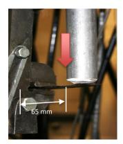
Figure 28: Experimental setup for flexural stiffness (courtesy of WSU).
