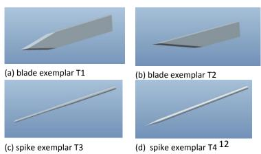
The tip and edge sharpness specifications of the exemplars was based on trials with different levels of material ground from the tips and edges until a match was found with the averaged push-through performance of each weapon style. Comparison of the exemplar performance from single tests to the average survey weapon subset
