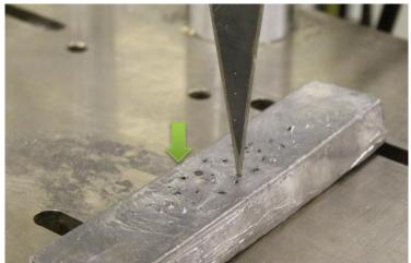
Figure 14: Tip sharpness indenter test setup.
