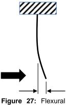
Figure 27: Flexural Stiffness
