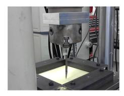
Figure 7: Push-through test.
