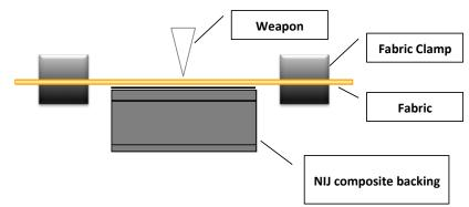
Figure 18: Push-through test components and setup
