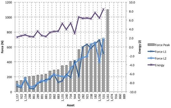
Figure 21: Push-through bladed weapon force test results.
