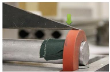
Figure 16: Edge sharpness test setup.
