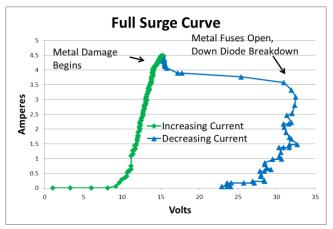
Figure 9: Full surge curve of a low capacitance device
