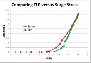
Figure 20: Comparing current versus voltage plots of a low capacitance device made using a 100 ns TLP with plots made using the surge stress
