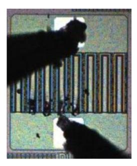
Figure 17: The 8 fingered device after 4 surge stresses
