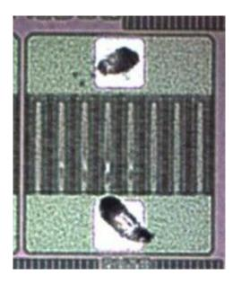
Figure 13: The 8 fingered device after 2 surge stresses
