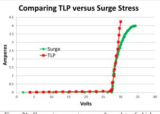
Figure 21: Comparing current versus voltage plots of a high voltage device made using a 100 ns TLP with plots made using the surge stress
