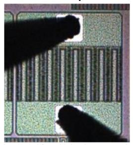
Figure 11: An 8 fingered device prior to surge stressing
