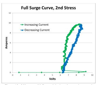
Figure 12: I-V curve of 8 fingered device taken on the second surge stress
