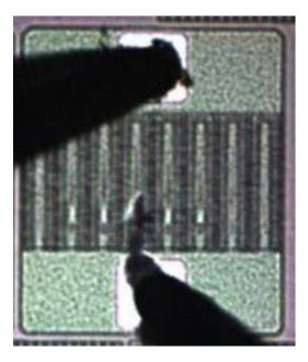
Figure 15: The 8 fingered device after 3 surge stresses
