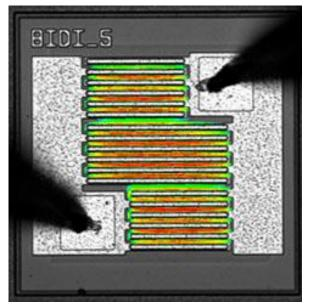
Figure 4: Current Distribution in a Bidirectional Zener diode. Stress is 2 mA DC.
