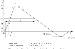
Figure 1: The Open Circuit Voltage Surge Pulse
