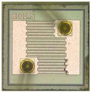
Figure 6: Damage in a Bidirectional Zener diode. Stress was 30 kV IEC 61000-4-2 ESD, same polarity as surge stress of Figure 5.
