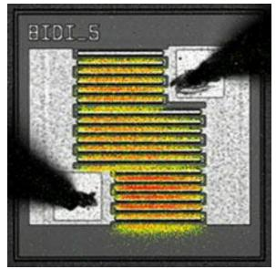
Figure 5: Current Distribution in a Bidirectional Zener diode. Stress is three 4 ampere pulses of IEC 61000-4-5 surge current.
