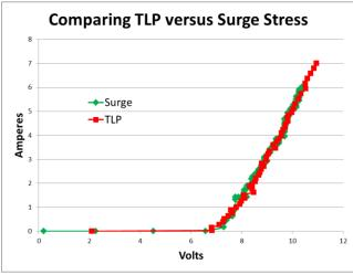
Figure 19: Comparing current versus voltage plots of a trench device made using a 100 ns TLP with plots made using the surge stress
