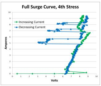
Figure 16: I-V curve of 8 fingered device taken on the fourth surge stress
