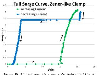
Figure 18: Current versus Voltage of Zener-like ESD Clamp Plotted during Surge Stress of 4.2 Amp Peak Current
