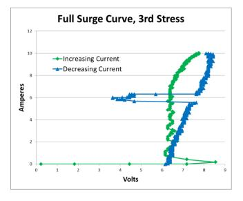
Figure 14: I-V curve of 8 fingered device taken on the third surge stress
