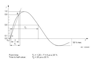
Figure 2: The Short Circuit Current Surge Pulse
