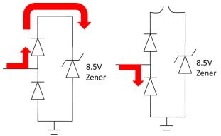
Figure 10: Current flow before and after metal failure
