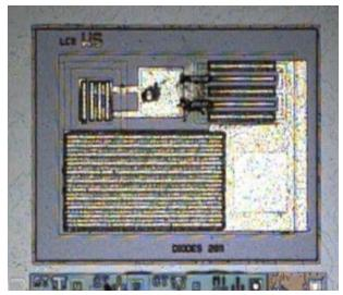
Figure 8: Photomicrograph of a low capacitance clamp stressed to failure using the surge pulse. Note the damage to the metal to the right of the top bond pad.
