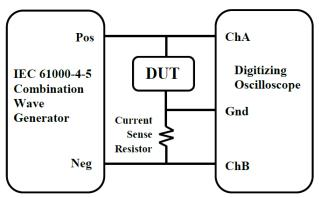
Figure 3: Test Setup Block Diagram
